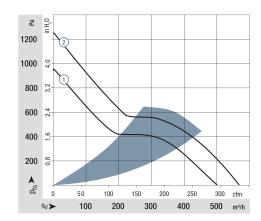
Air performance measured according to: ISO 5801. Installation category A, without contact protection. Noise: Total sound power level  $L_WA$  ISO 103002 measured on a hemisphere with a radius of 2 m. Sound pressure level  $L_pA$  measured at 1 m distance from fan axis.
