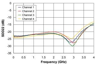
FIGURE 20. OUTPUT DIFFERENTIAL RETURN LOSS
