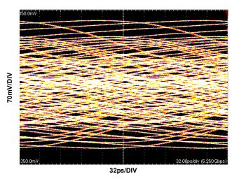
FIGURE 13. RECEIVED SIGNAL AFTER 15m OF 28AWG TWIN-AXIAL CABLE (CABLE D) (Note 18), 6.25 Gb/s
