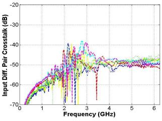
FIGURE 21. DIFFERENTIAL CROSSTALK BETWEEN ADJACENT INPUT CHANNEL
