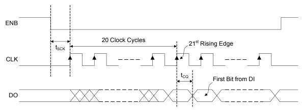
FIGURE 30. TIMING DIAGRAM FOR DI/DO CARRYOVER
