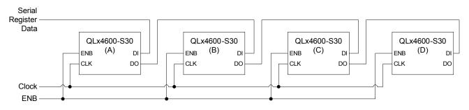
FIGURE 31. SERIAL BUS PROGRAMMING MULTIPLE QLX4600-S30 DEVICES USING DI/DO CARRYOVER
