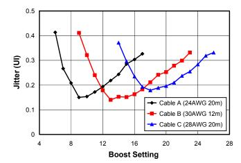
FIGURE 4A. JITTER vs CABLE LENGTH, 5Gb/s
