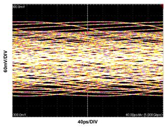
FIGURE 7. RECEIVED SIGNAL AFTER 12m OF 30AWG TWIN-AXIAL CABLE (CABLE B), 5Gb/s
