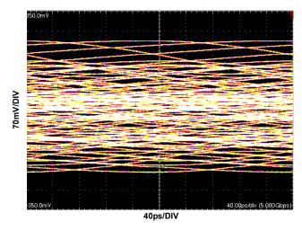
FIGURE 11. RECEIVED SIGNAL AFTER 30m OF 24AWG TWIN-AXIAL CABLE (Note 18), 5Gb/s
