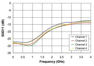
FIGURE 19. INPUT DIFFERENTIAL RETURN LOSS
