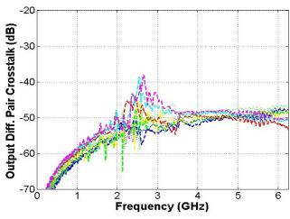
FIGURE 22. DIFFERENTIAL CROSSTALK BETWEEN ADJACENT INPUT CHANNELS
