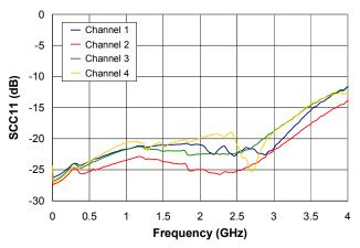
FIGURE 17. INPUT COMMON-MODE RETURN LOSS
