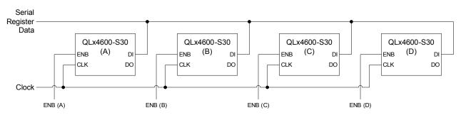
FIGURE 29. SERIAL BUS PROGRAMMING MULTIPLE QLX4600-S30 DEVICES USING SEPARATE ENB SIGNALS
