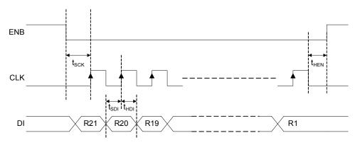
FIGURE 28. TIMING DIAGRAM FOR PROGRAMMING THE INTERNAL REGISTERS OF THE QLX4600-S30
