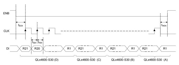
FIGURE 32. TIMING DIAGRAM FOR PROGRAMMING MULTIPLE QLX4600-S30 DEVICES USING DI/DO CARRYOVER
