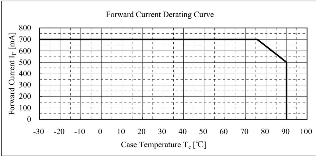
(Note) To keep the case temperature lower than the rating, enough heat-radiation performance needs to be secured by using an adequate heat sink.
