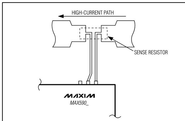
Figure 14. Kelvin Connection for the Current-Sense Resistors
