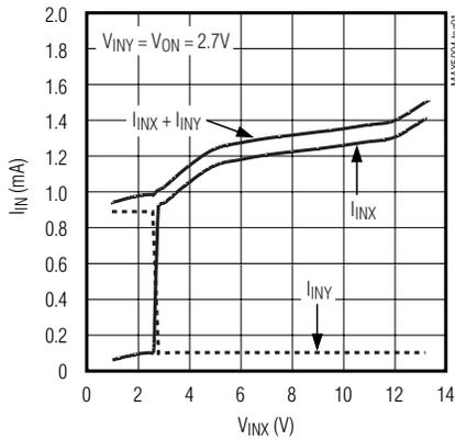
**TOTAL SUPPLY CURRENT vs. SUPPLY VOLTAGE**
