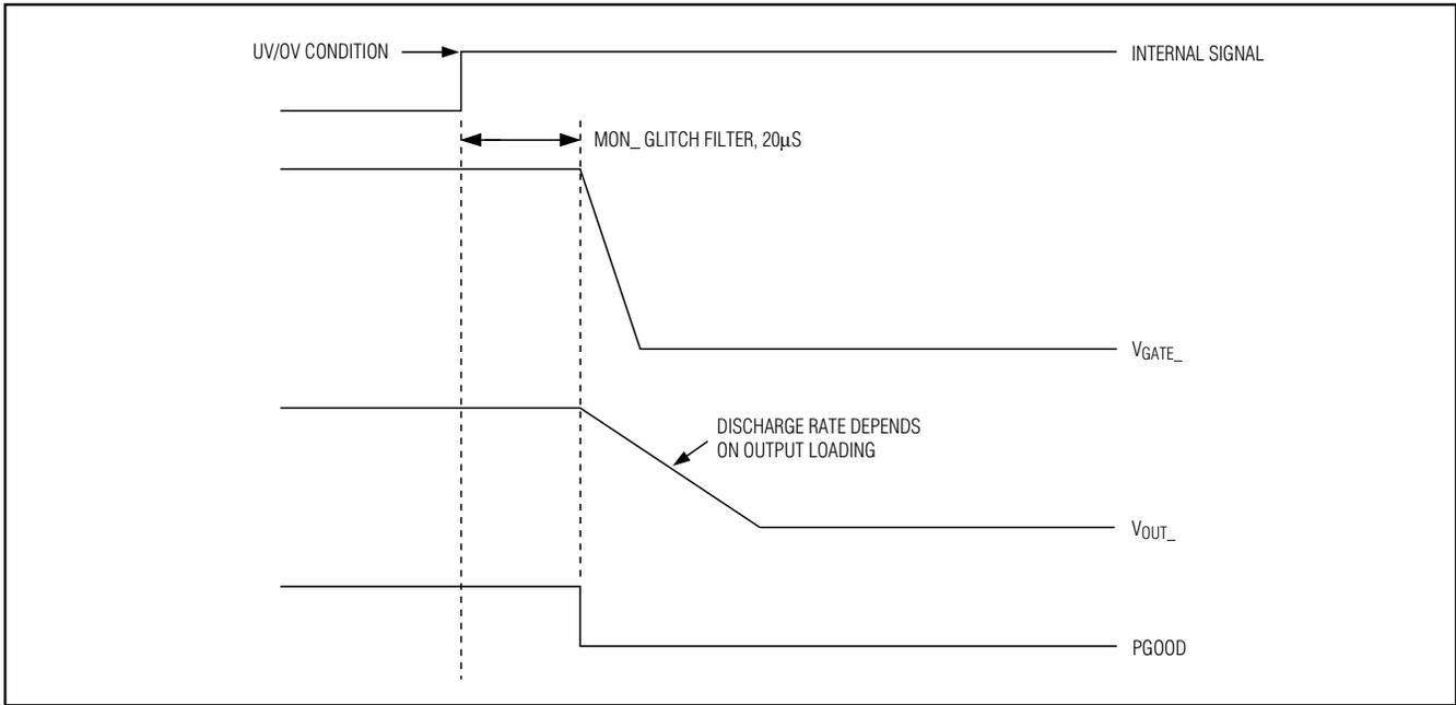
Figure 6. Power-Down when an Undervoltage/Overvoltage Fault Occurs (MAX5906/MAX5907)
