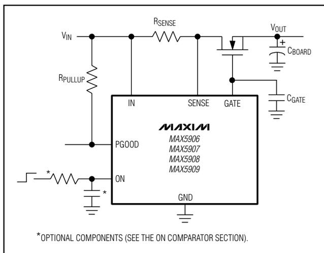
Figure 10. Operating with an External Gate Capacitor
