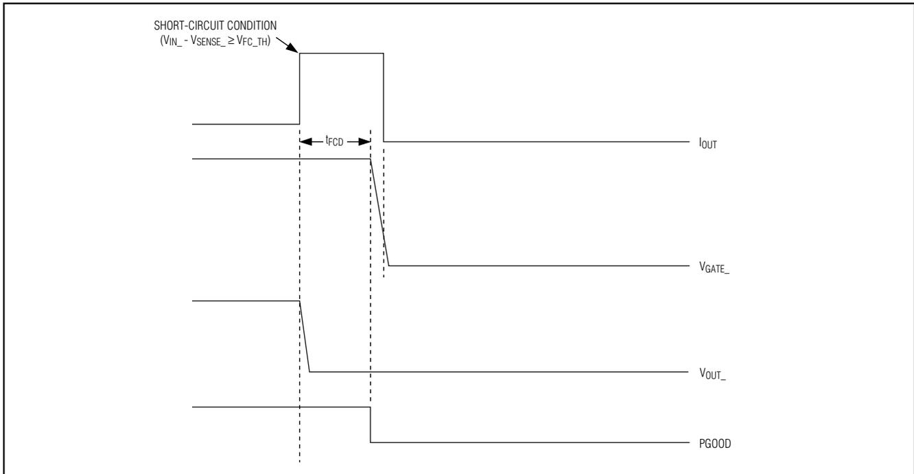
Figure 5. Power-Down when a Short-Circuit Fault Occurs
