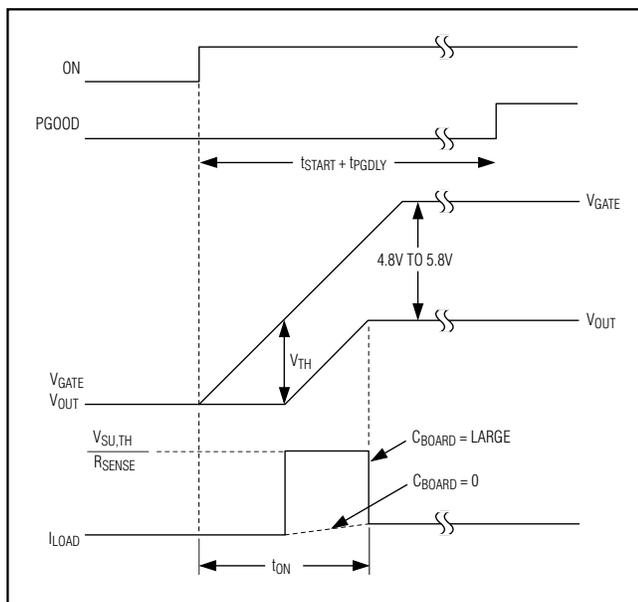
Figure 2. Startup Waveforms
