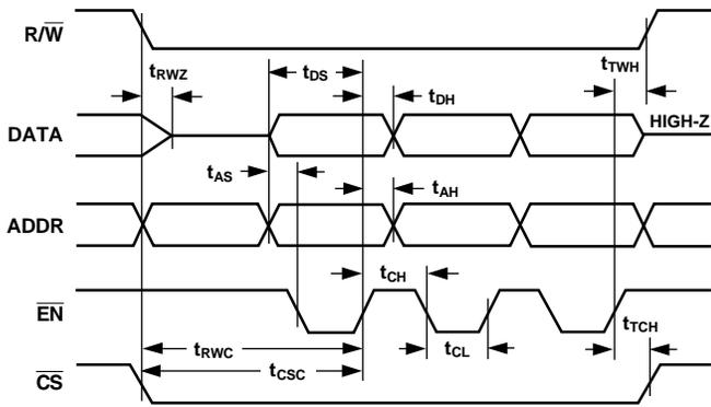
Figure 2. Write Timing
