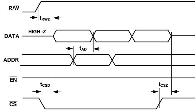
Figure 3. Readback Timing
