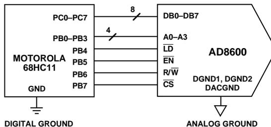
Figure 21. Interfacing the 68HC11 to the AD8600
