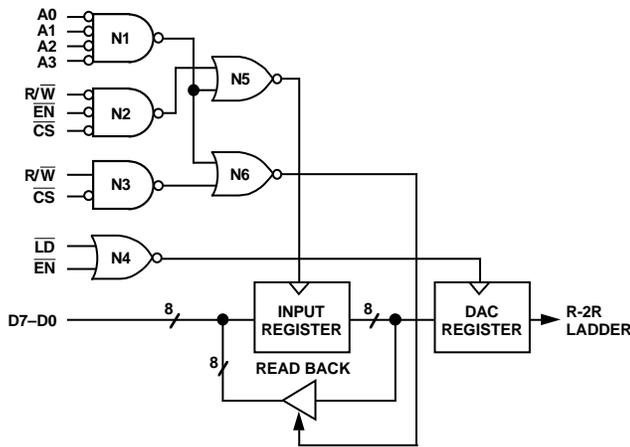
Figure 19. Logic Interface Circuit for DAC Channel 0
