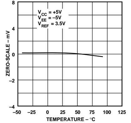
Figure 7. Zero-Scale Voltage vs. Temperature
