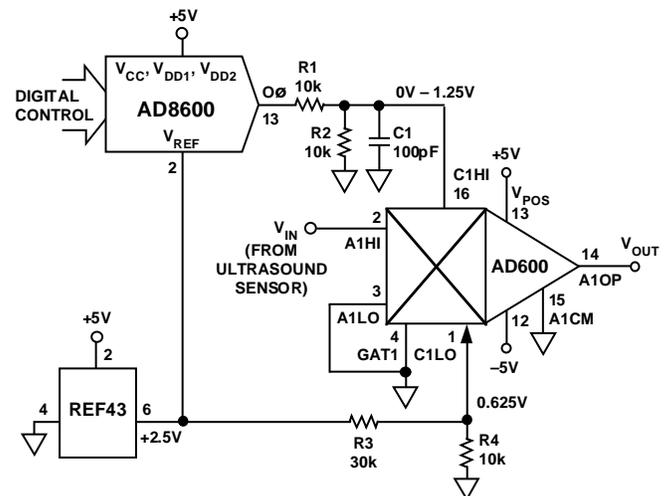
Figure 23. Ultrasound Amplifier with Digitally Controlled Variable Gain
