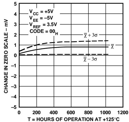
Figure 15. Output Voltage Drift Accelerated by Burn-In
