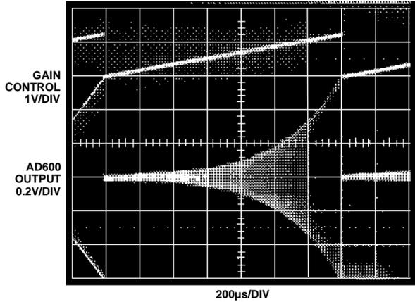
Figure 24. Time Dependent Gain of the AD600
