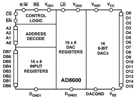
At system power up or during fault recovery the reset ( $\overline{RS}$ ) pin forces all DAC registers into the zero state which places zero volts at all DAC outputs.
