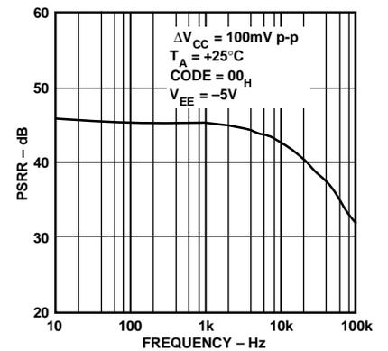
Figure 13. PSRR vs. Frequency
