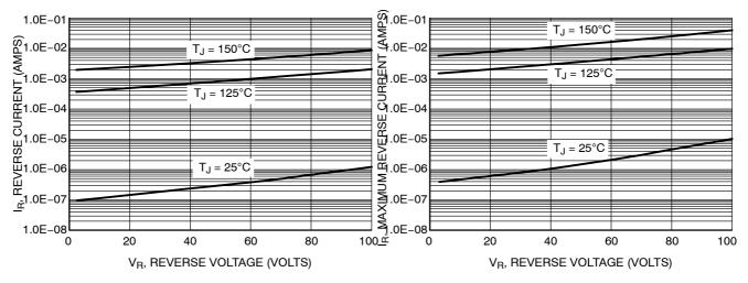
Figure 3. Typical Reverse Current
