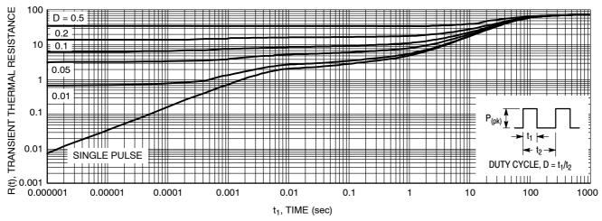
Figure 8. Thermal Response Junction-to-Ambient
