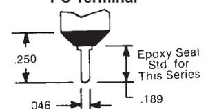
**Sensitive Snap-Action Pushbutton Switches — Solder and P.C. Terminals (Momentary Action)**
