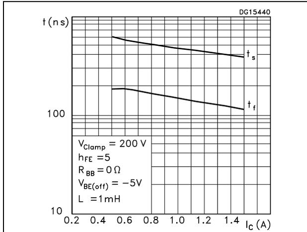
Figure 14. Resistive load storage time PNP
