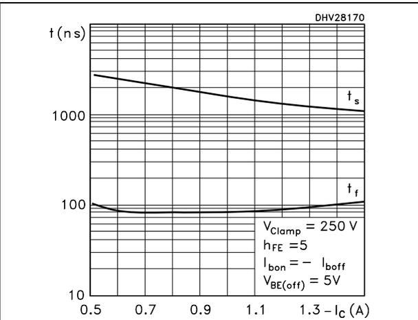
Figure 13. Resistive load storage time NPN
