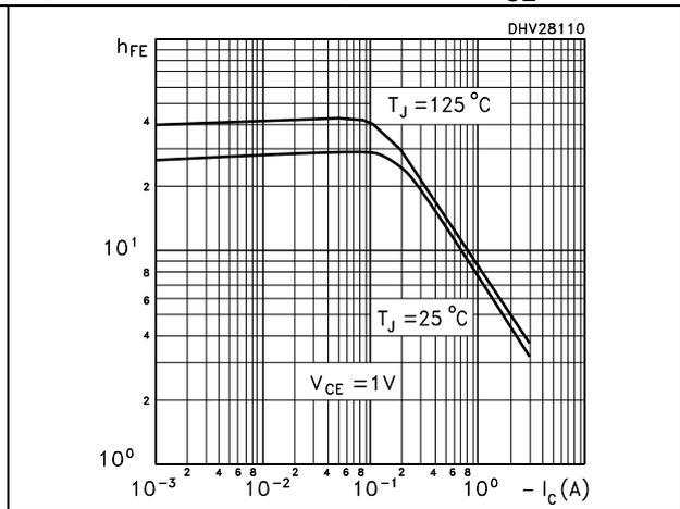
Figure 4. DC current gain NPN ( $V_{CE} = 1\text{ V}$ )
