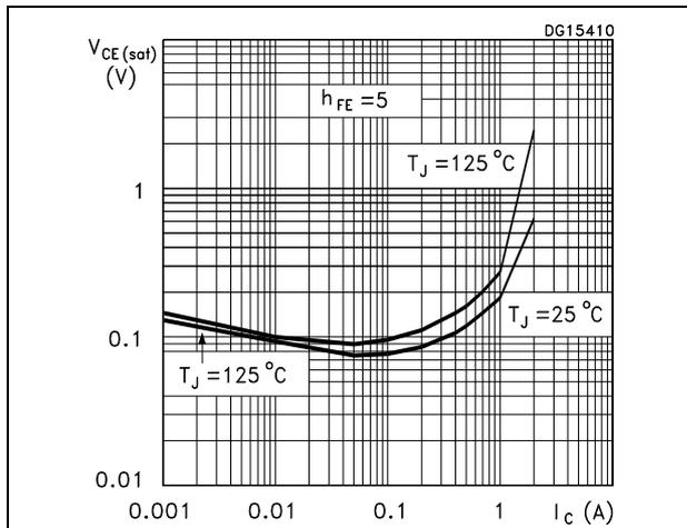
Figure 8. Collector emitter saturation voltage PNP
