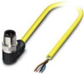
Sensor/Actuator cable, 4-position, TPE, Plug angled M12 SPEEDCON, A-coded, on free cable end, Cable length: 2 m
