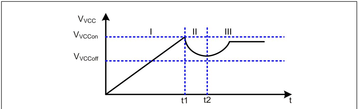
Figure 4 VCC voltage at start up
