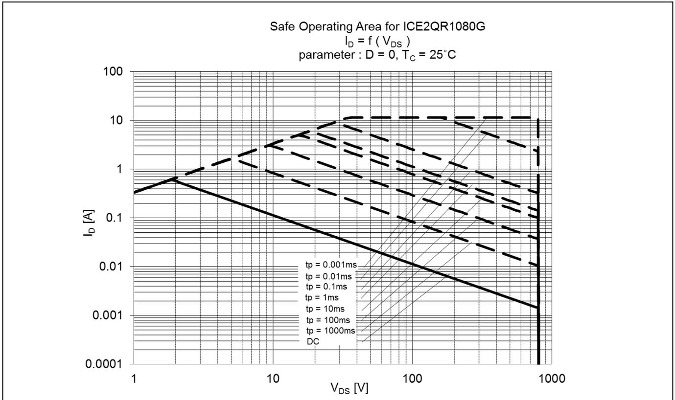
Figure 10 Safe Operating Area (SOA) curve for ICE2QR1080G
