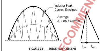
$$\begin{split} &I_{\text{IN(t)}} &= \sum &\text{AVE [I_L (t)]} \\ &I_{\text{IN}} &= \frac{1}{T} \left[ \frac{\left( I_L \right) \ \left( T \right)}{2} \right] = \frac{I_L}{2} \\ &I_{\text{INpeak}} = I_P = \frac{I_{\text{LP}}}{2} \end{split}$$
