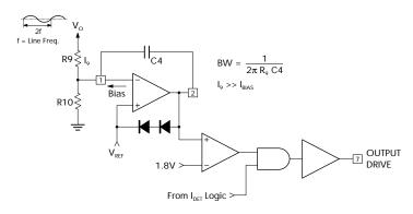
FIGURE 27 — THE AMPLIFIER CONFIGURED AS AN INTEGRATOR FOR LOOP COMPENSATION
