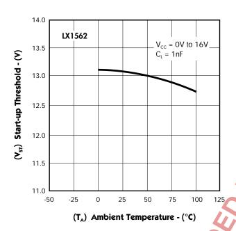
FIGURE 10. — START-UP THRESHOLD vs. TEMPERATURE
