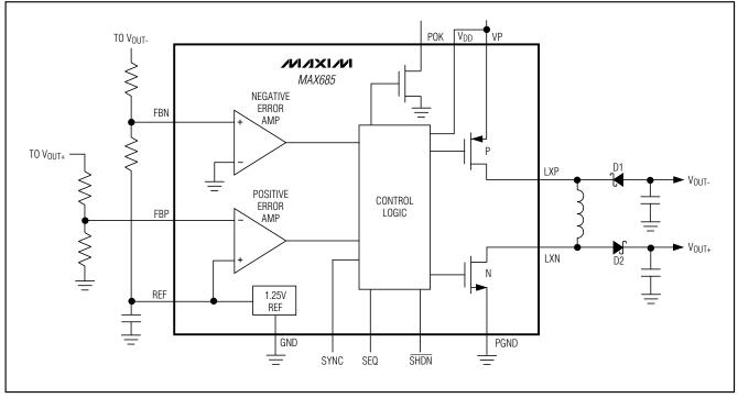
Figure 1. Functional Diagram
