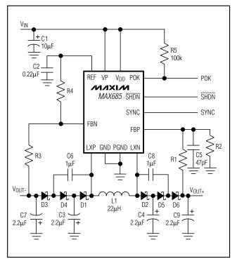
Figure 4. Circuit for Output Voltages < -9V and > +24V
