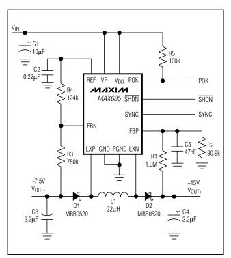
Figure 3. Standard Application Circuit
