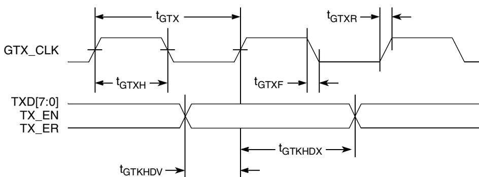
**Figure 10. GMII Transmit AC Timing Diagram****8.2.2.2 GMII Receive AC Timing Specifications**
