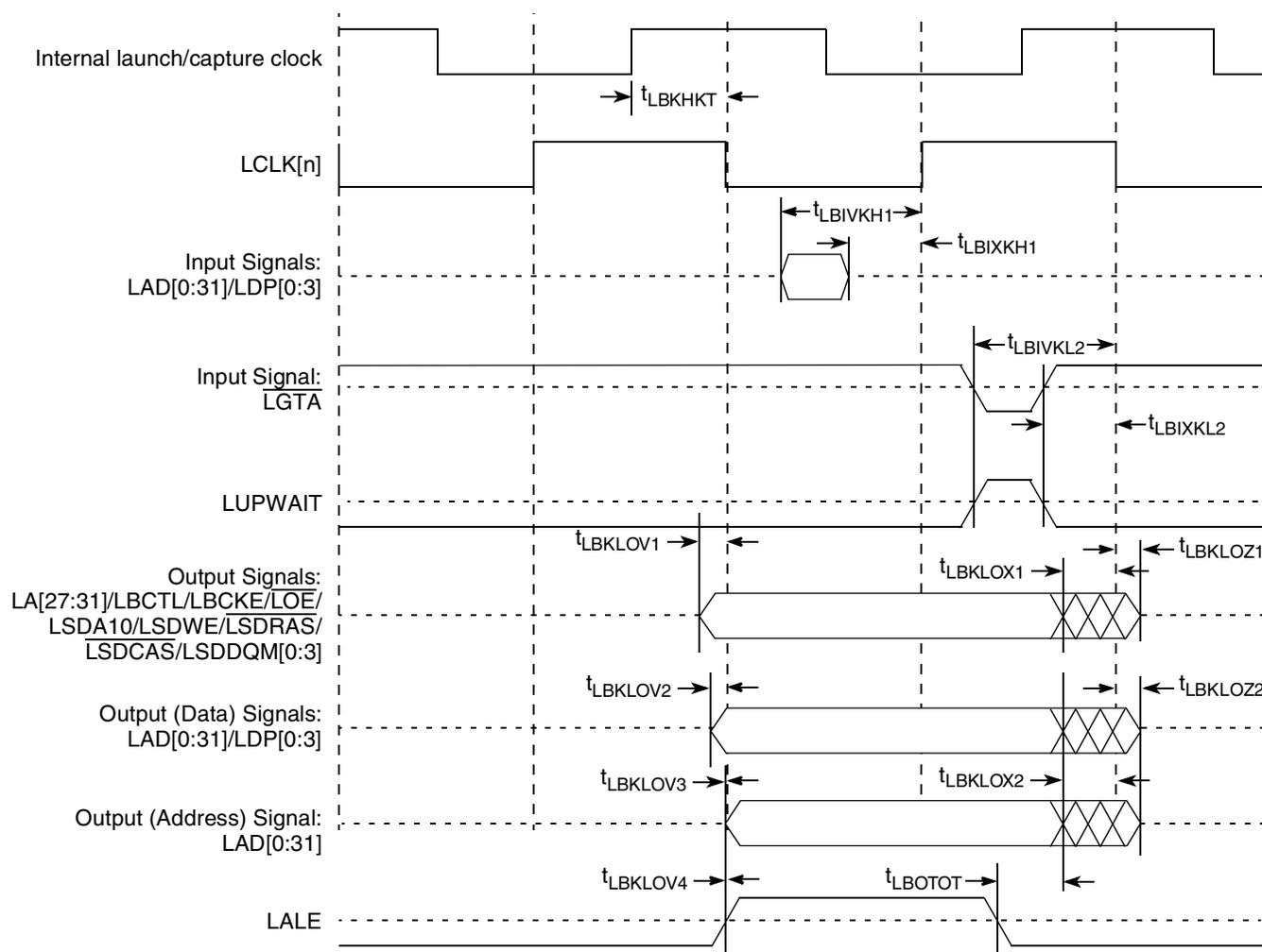
Figure 27. Local Bus Signals (PLL Bypass Mode)
