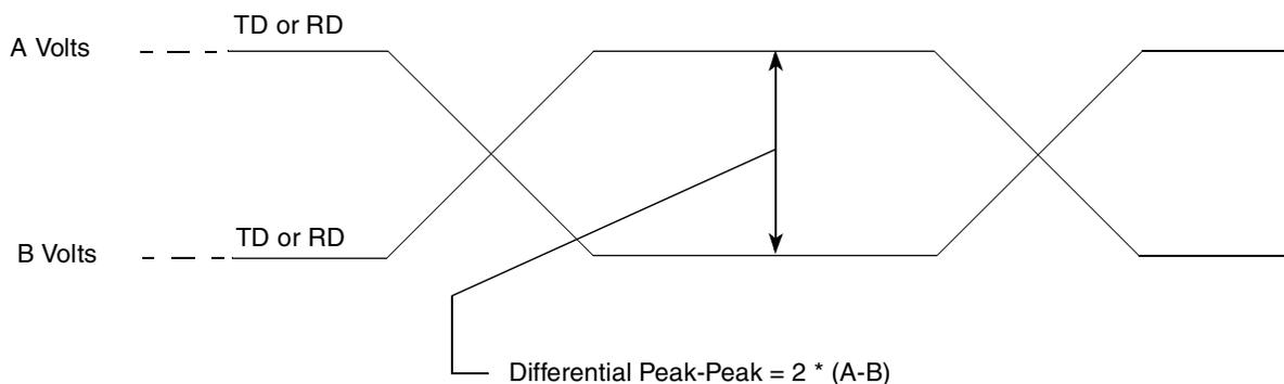
Figure 53. Differential Peak-Peak Voltage of Transmitter or Receiver
