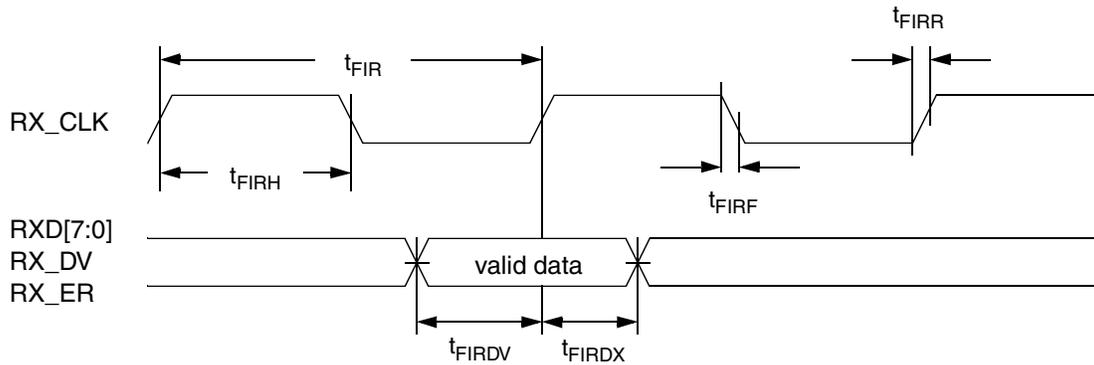
Figure 9. FIFO Receive AC Timing Diagram
