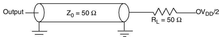
**Figure 36. I<sup>2</sup>C AC Test Load**
