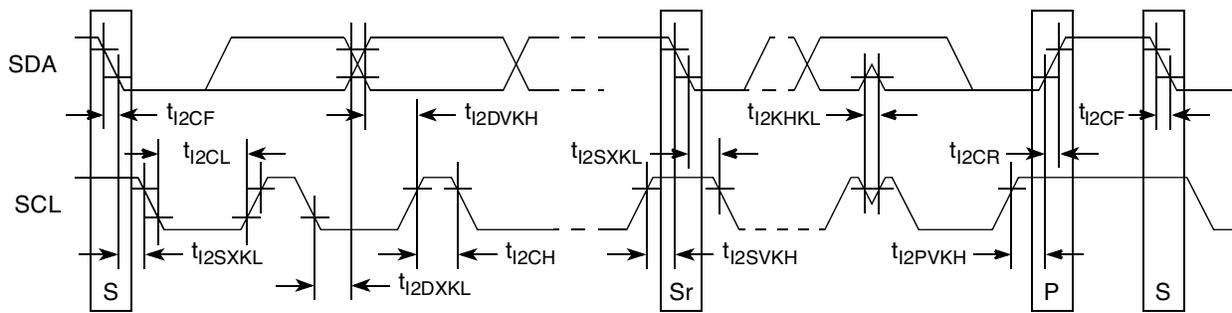
Figure 37. I<sup>2</sup>C Bus AC Timing Diagram
