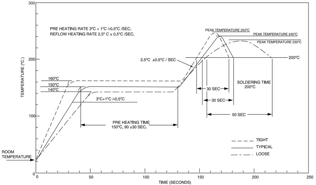
For leaded (Pb) parts, the peak temperature shown in this profile can be decreased to as low as  $230^{\circ}\text{C}$ . Exceeding  $265^{\circ}\text{C}$  at peak or the time at peak temperature shown in this profile can damage the parts. Specifically:
