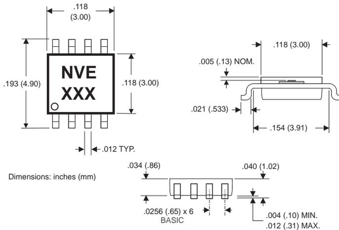
**Note:** MSOP8 Package has thermal power dissipation of 320°C/Watt in free air. Attaching the package to a circuit board improves thermal performance.
