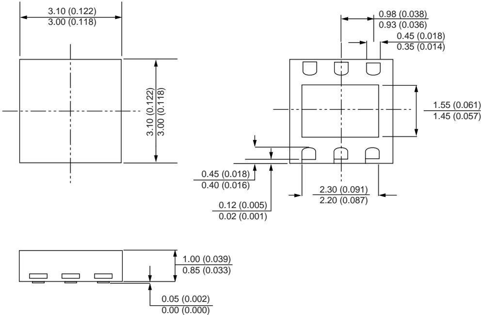
**Note:** The PLLP6 package has thermal power dissipation of 320°C/Watt in free air. Attaching the package to a circuit board improves thermal performance. Dimensions are in mm (inches).
