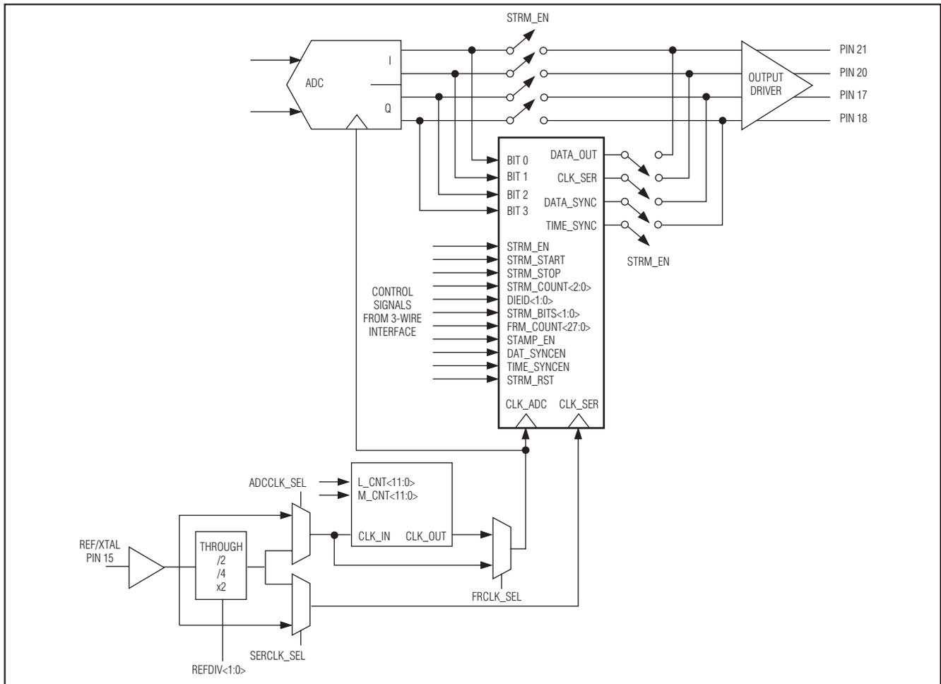
Figure 3. DSP Interface Top-Level Connectivity and Control Signals
