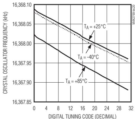
**CRYSTAL OSCILLATOR FREQUENCY VARIATION vs. TEMPERATURE**
