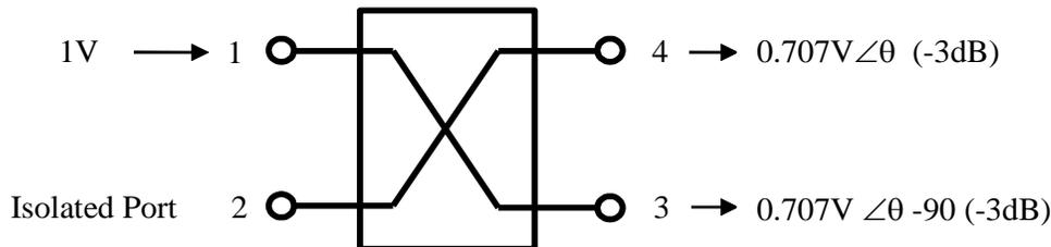
The hybrid coupler can also be used to combine two signals that are applied with equal amplitudes and phase quadrature ( $90^\circ$  phase difference). An example of this function is illustrated below.
