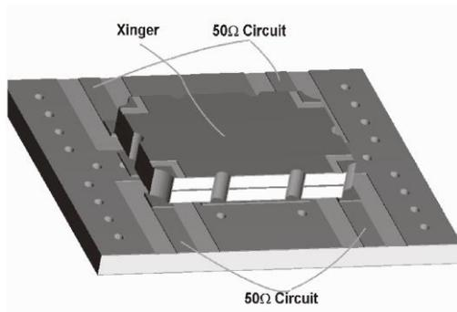
**Figure 3: Component Placement**
