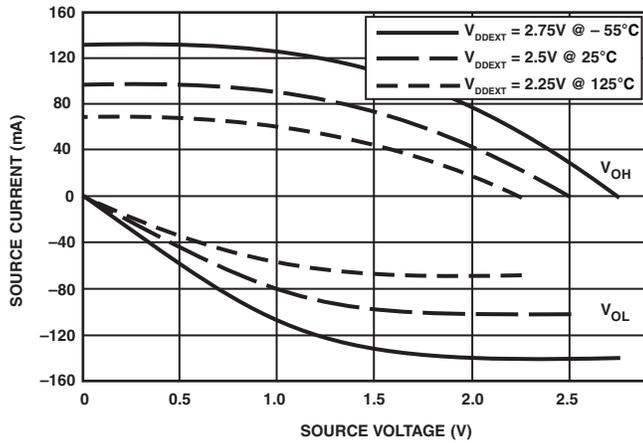
Figure 33. Driver Type B Current (2.5 V  $V_{DDEXT}$ )
