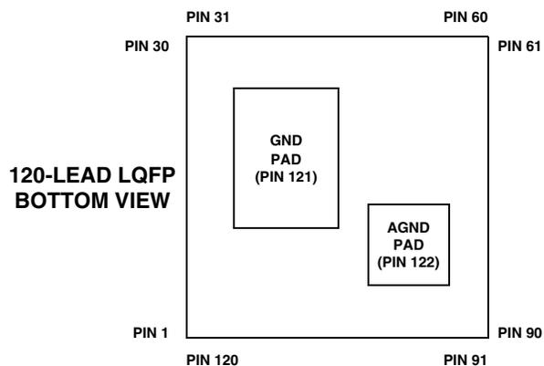
Figure 90. 120-Lead LQFP Package Lead Configuration (Bottom View)
