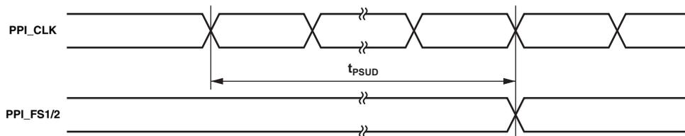
Figure 13. PPI with External Frame Sync Timing
