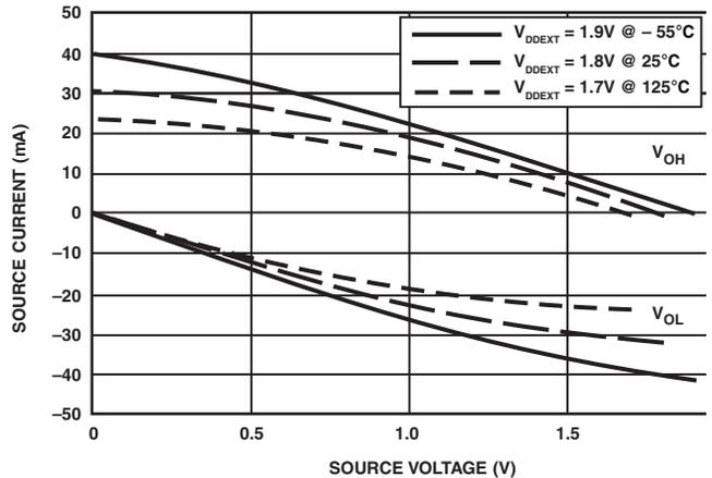
Figure 37. Driver Type C Current (1.8 V  $V_{DDEXT}$ )
