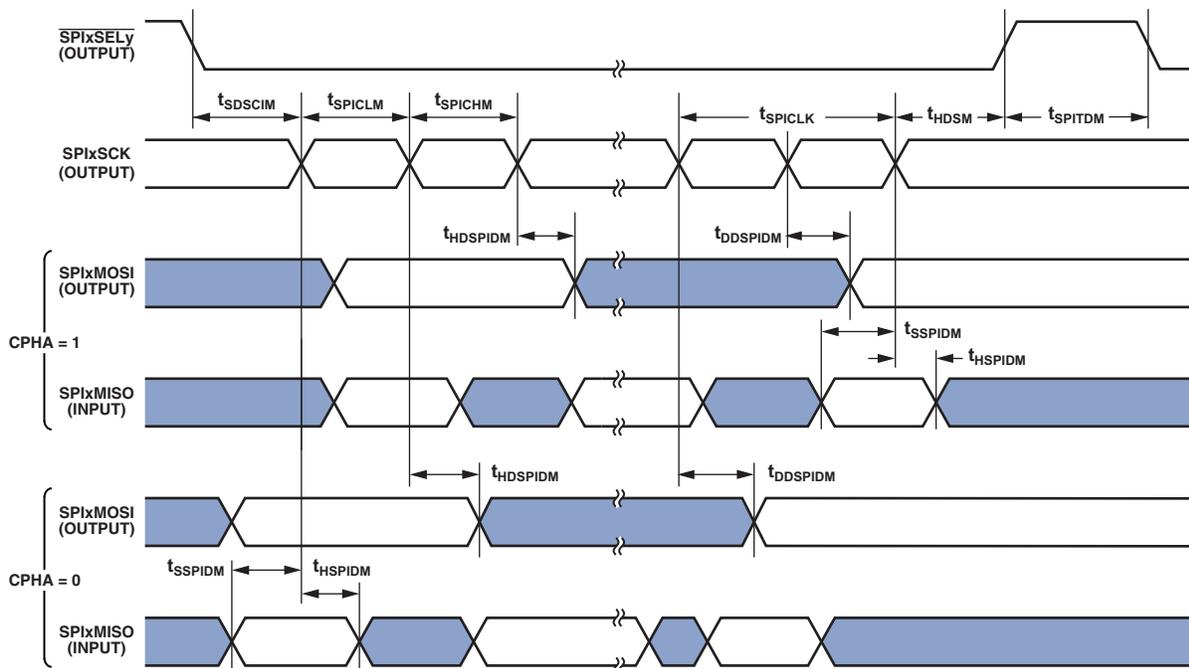
Figure 23. Serial Peripheral Interface (SPI) Port—Master Timing
