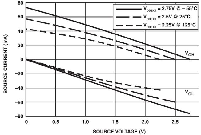
Figure 36. Drive Type C Current (2.5 V  $V_{DDEXT}$ )
