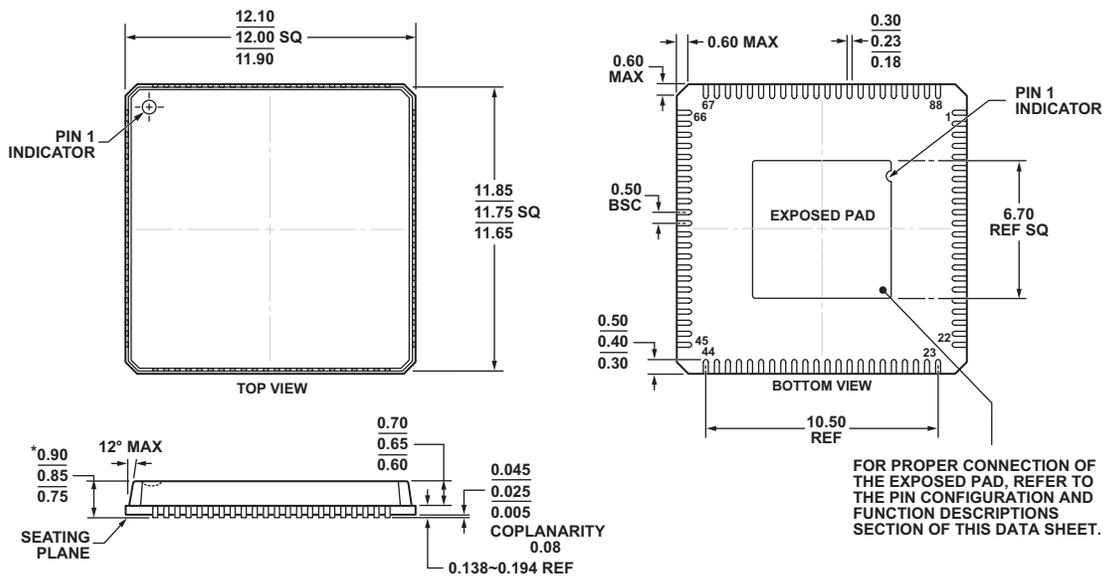
\*COMPLIANT TO JEDEC STANDARDS MO-220-VRRD EXCEPT FOR MINIMUM THICKNESS AND LEAD COUNT.
