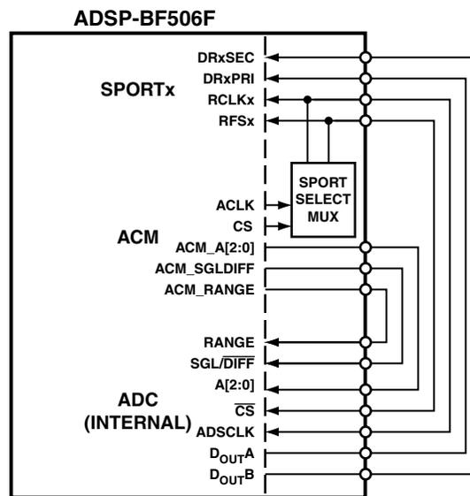
Figure 7. ADC (Internal), ACM, and SPORT Connections
