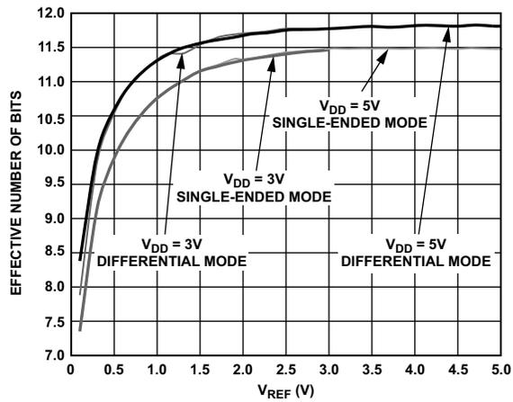
Figure 57. Effective Number of Bits vs.  $V_{REF}$
