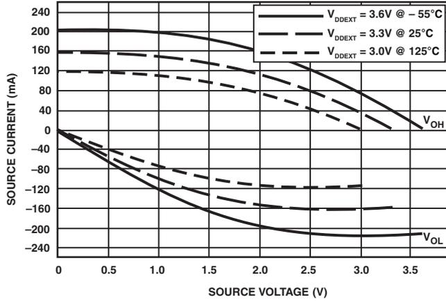
Figure 32. Driver Type B Current (3.3 V  $V_{DDEXT}$ )
