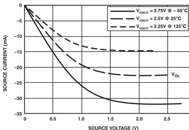
Figure 39. Driver Type D Current (2.5 V  $V_{DDEXT}$ )
