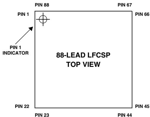
Figure 91. 88-Lead LFCSP Lead Configuration (Top View)
