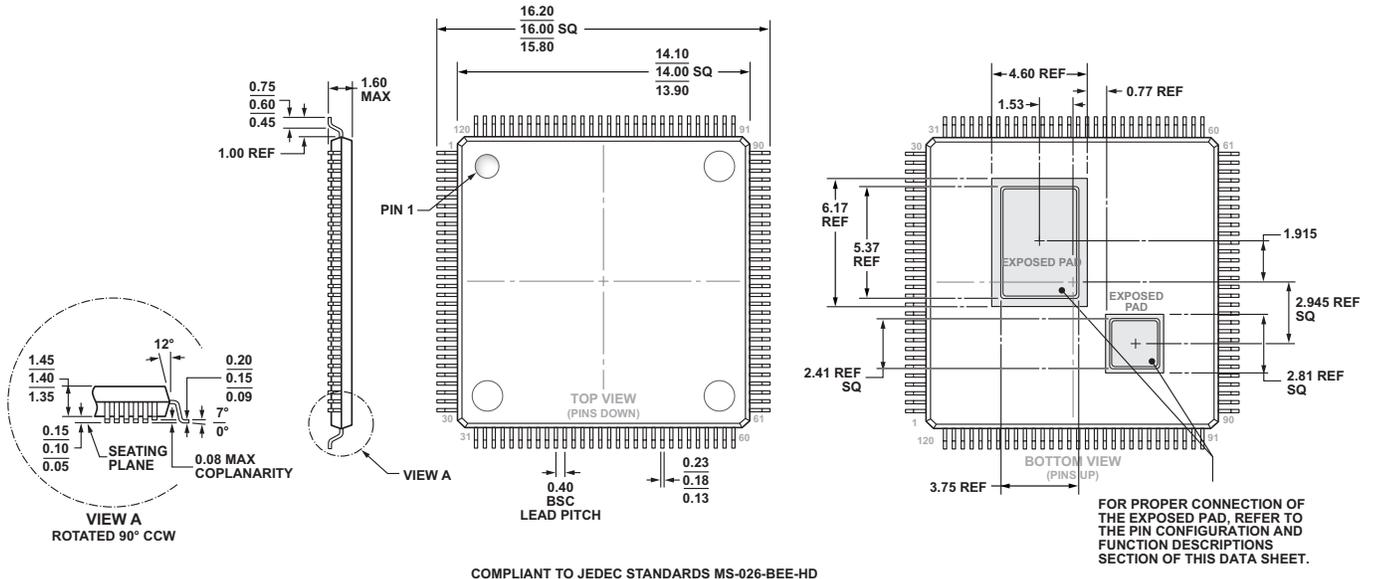
*Figure 93. 120-Lead Low Profile Quad Flat Package, Exposed Pad [LQFP\_EP]<sup>1</sup>
