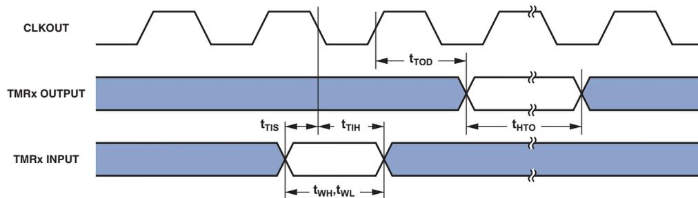
Figure 26. Timer Cycle Timing
