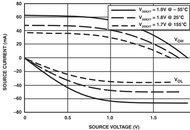
Figure 34. Driver Type B Current (1.8 V  $V_{DDEXT}$ )
