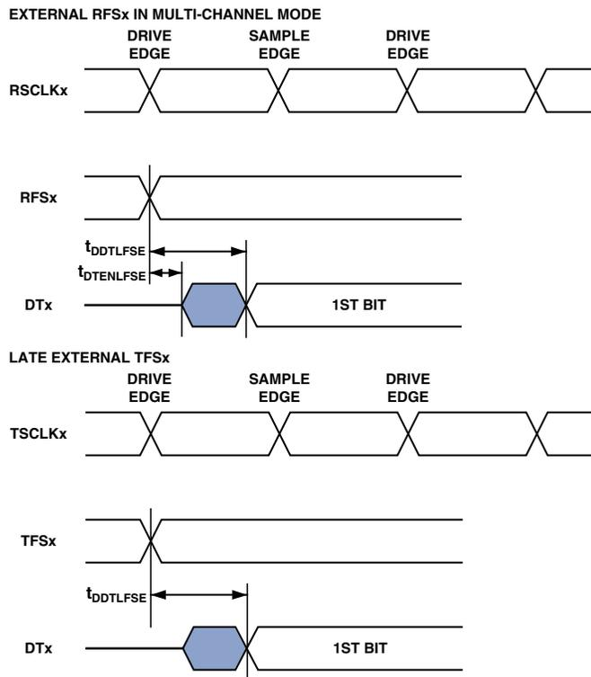
Figure 22. Serial Ports — External Late Frame Sync
