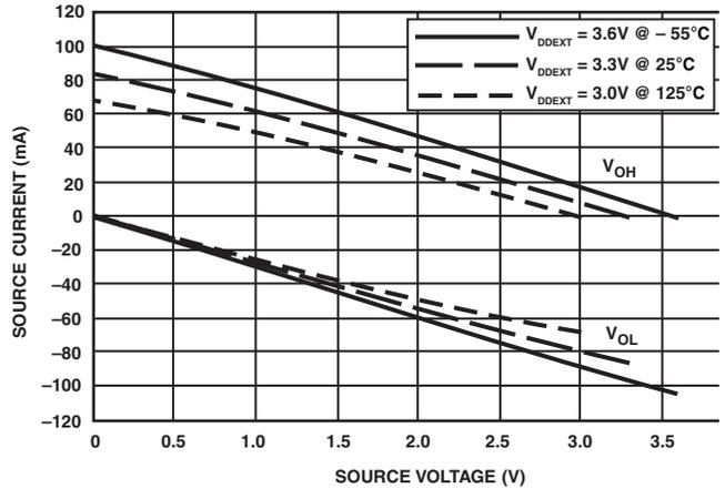
Figure 35. Driver Type C Current (3.3 V  $V_{DDEXT}$ )
