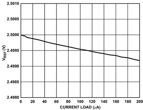
Figure 58.  $V_{REF}$  vs. Reference Output Current Drive
