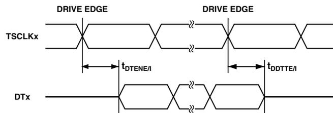
Figure 21. Serial Ports — Enable and Three-State
