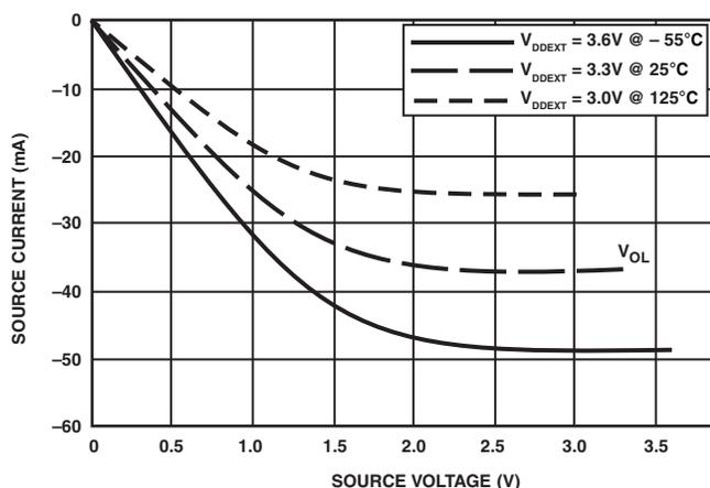
Figure 38. Driver Type D Current (3.3 V  $V_{DDEXT}$ )
