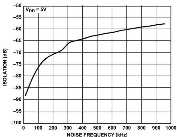
Figure 51. Channel-to-Channel Isolation
