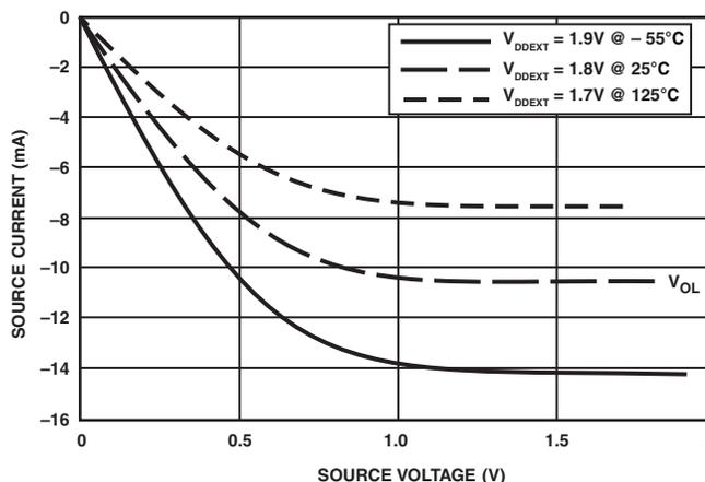
Figure 40. Driver Type D Current (1.8 V  $V_{DDEXT}$ )
