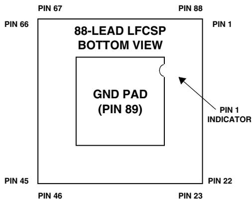
Figure 92. 88-Lead LFCSP Lead Configuration (Bottom View)
