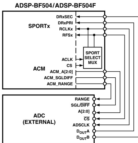
Figure 6. ADC (External), ACM, and SPORT Connections
