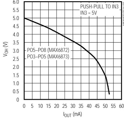
**OUTPUT VOLTAGE HIGH vs. SOURCE CURRENT (CHARGE-PUMP OUTPUT)**
