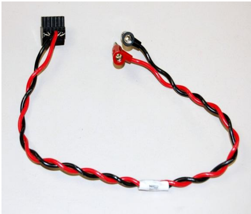
Figure 3: Power supply to driver board cable
