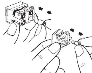
Note: Built-in LEDs cannot be replaced.
