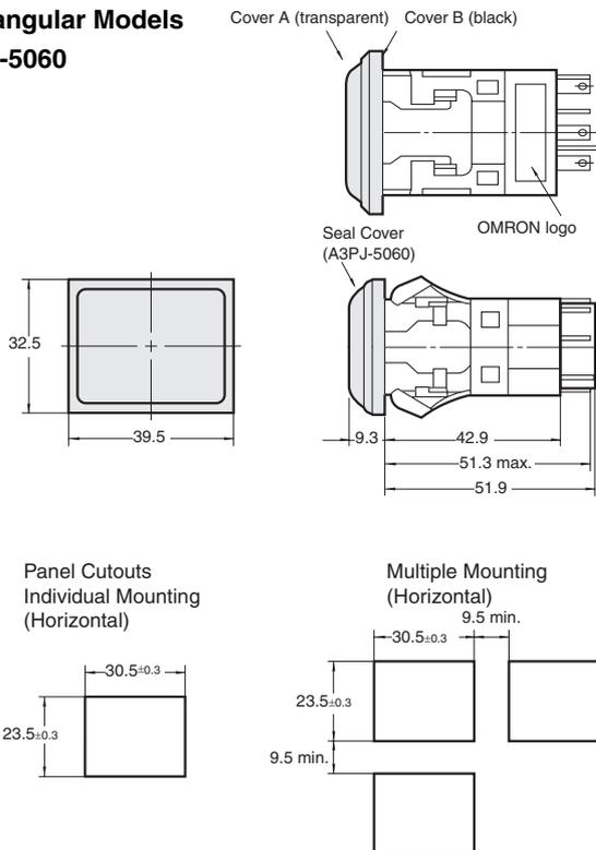
Note: 1. Recommended panel thickness: 1 to 5 mm
