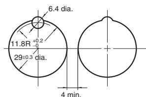
Note: 1. Recommended panel thickness: 1 to 5 mm
