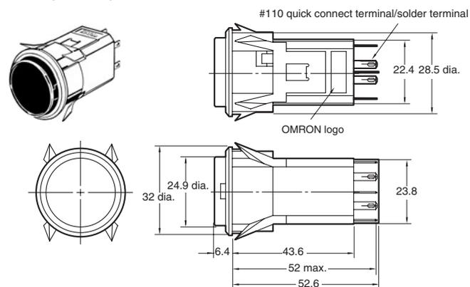
Note: The thickness of tab terminals #110 and solder terminals is 0.5 mm.
