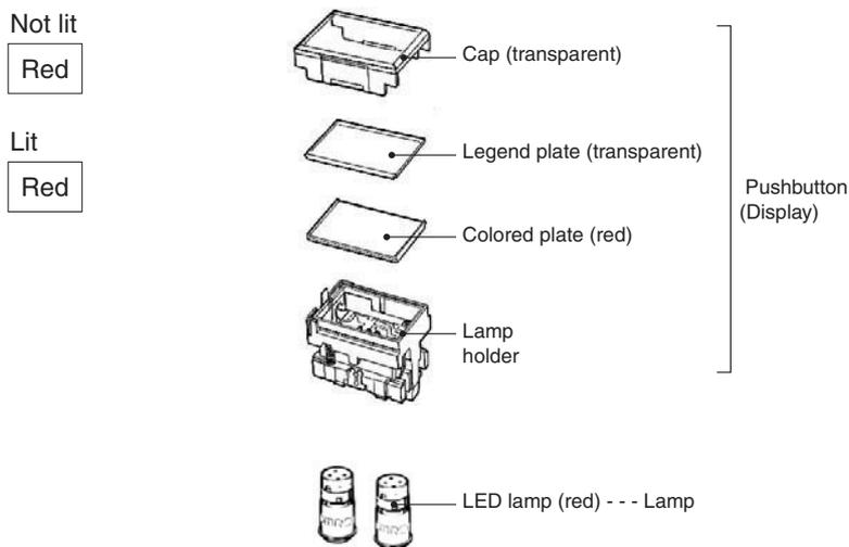
“Colored illumination” describes LED models for which the screen color is white when the LED is not lit and changes to the color of the LED lamp when the LED is lit.
