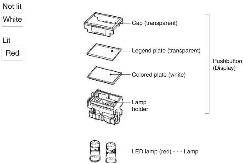
**Ordering: With colored-illumination models, order the Pushbutton, Lamp, and Switch as shown in the following table.**
