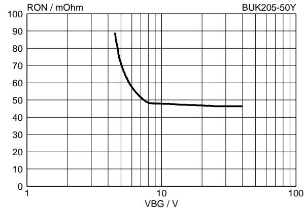
Fig.8. Typical on-state resistance,  $T_j = 25^\circ\text{C}$ .
