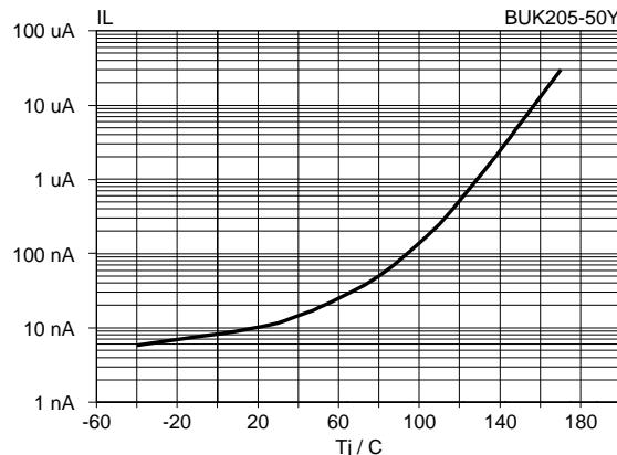
Fig.13. Typical off-state leakage current.
