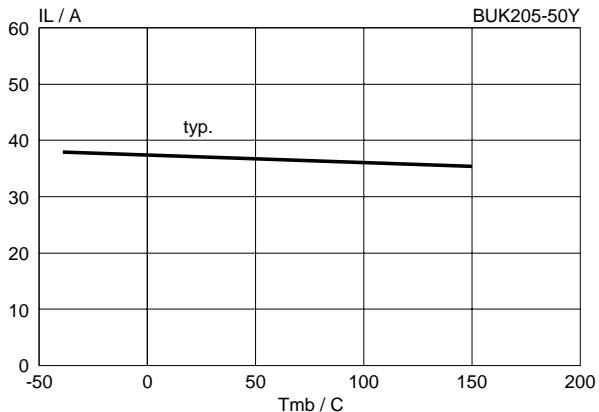
Fig.34. Typical overload current,  $V_{BL} = 9$  V.
