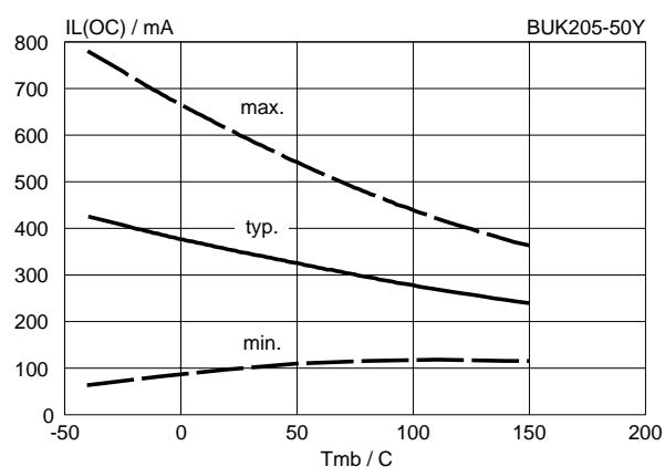
Fig.23. Low load current detection threshold,  $I_{L(OC)} = f(T_j)$ ; conditions  $V_{IG} = 5 V$ ;  $V_{BG} = 13 V$
