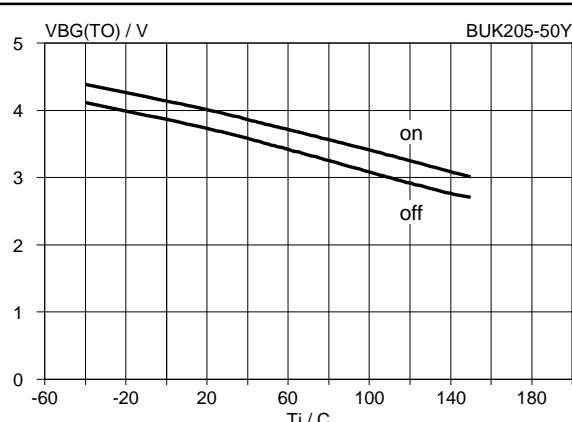
Fig.24. Supply typical undervoltage thresholds,  $V_{BG(TO)} = f(T_j)$ ; conditions  $V_{IG} = 3 V$ ;  $I_L = 80 mA$
