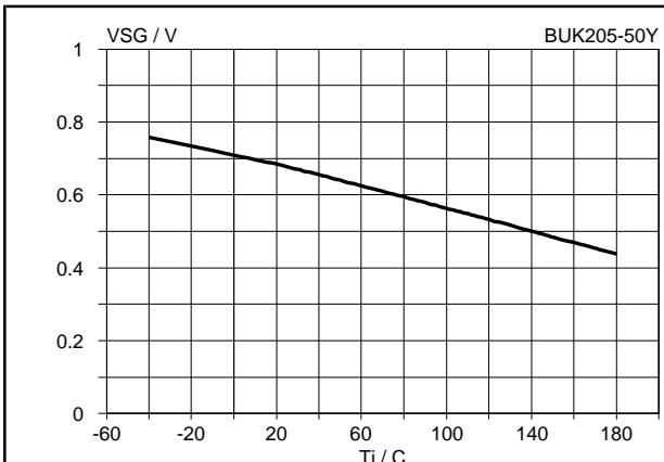
Fig.21. Typical status low voltage,  $V_{SG} = f(T_j)$ .
