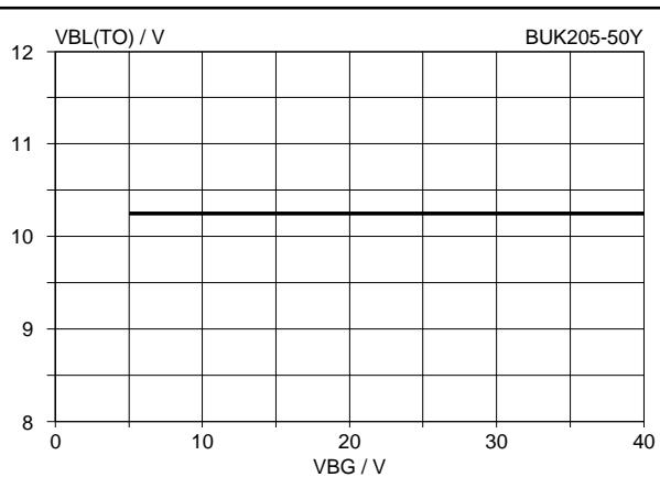
Fig.35. Typical short circuit load threshold voltage.
