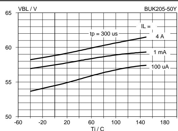
Fig.29. Typical battery to load clamping voltage.
