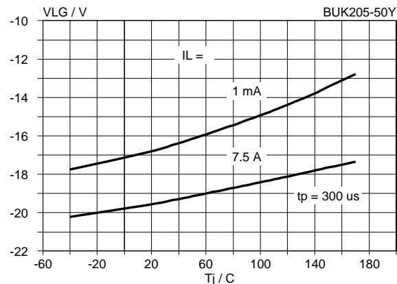
Fig.28. Typical negative load clamping voltage.
