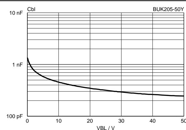
Fig.32. Typical output capacitance.  $T_{mb} = 25$  °C
