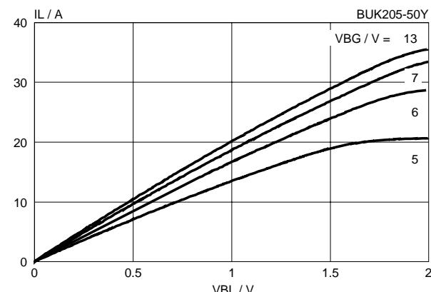
Fig.7. Typical on-state characteristics,  $T_j = 25^\circ\text{C}$ .
