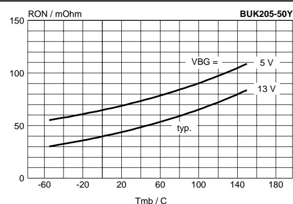
Fig.9. Typical on-state resistance,  $t_p = 300\ \mu\text{s}$ .
