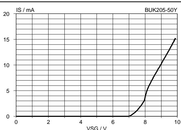
Fig.18. Typical status characteristic,  $T_j = 25$  °C.
