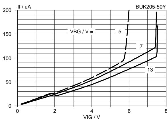
Fig.14. Typical input characteristics,  $T_j = 25\text{ °C}$ .
