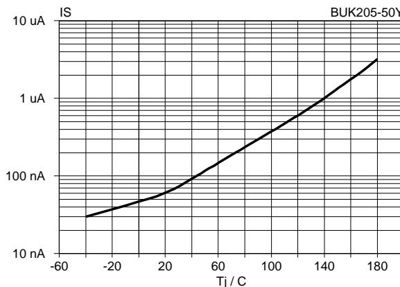
Fig.19. Typical status leakage current.
