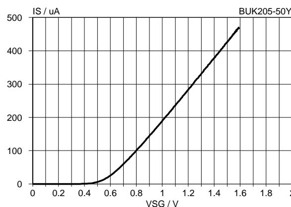
Fig.20. Typical status low characteristic,  $T_j = 25$  °C.
