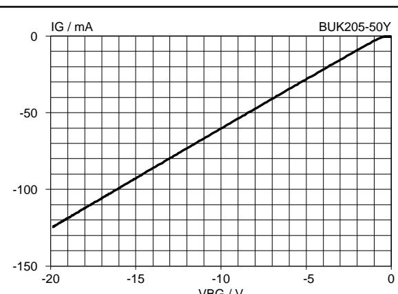
Fig.30. Typical reverse battery characteristic.
