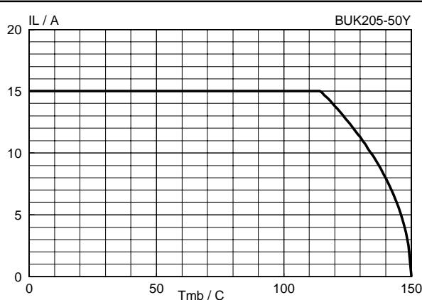
Fig.6. Limiting continuous on-state load current.
