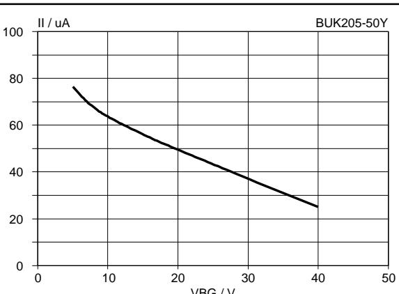
Fig.15. Typical input current,  $T_j = 25\text{ °C}$ .
