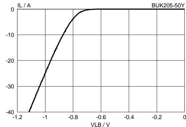
Fig.31. Typical reverse diode characteristic.
