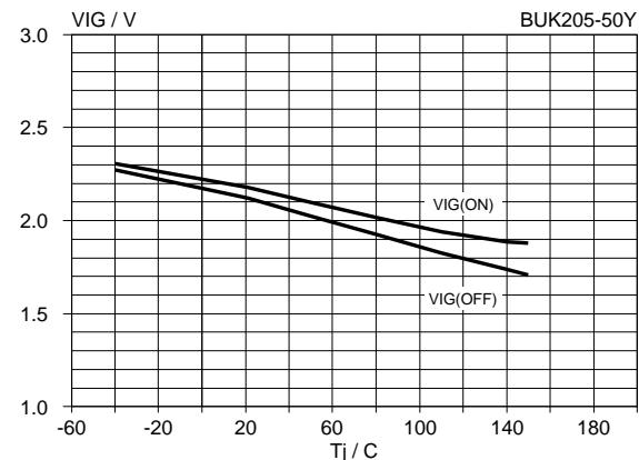
Fig.16. Typical input threshold voltages.
