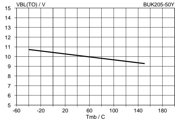
Fig.36. Typical short circuit load threshold voltage.
