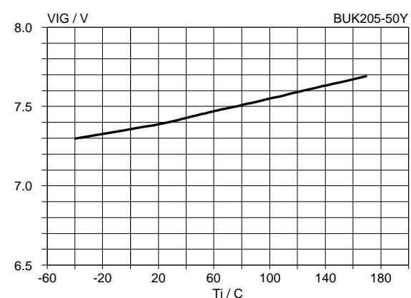
Fig.17. Typical input clamping voltage.
