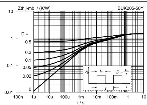
Fig.37. Transient thermal impedance.
