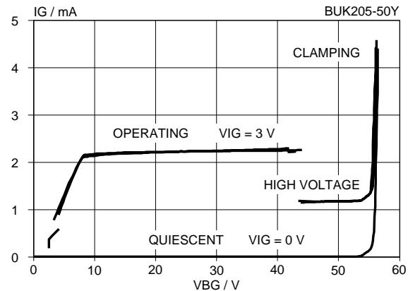
Fig.10. Typical supply characteristics, 25 °C.
