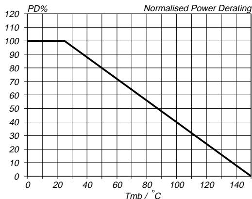
Fig.5. Normalised limiting power dissipation.
