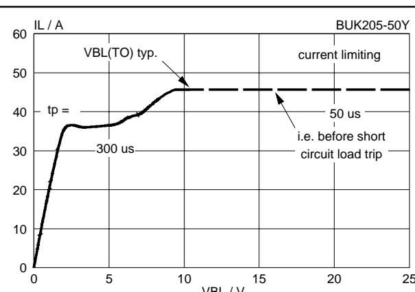
Fig.33. Typical overload characteristic,  $T_{mb} = 25$  °C.
