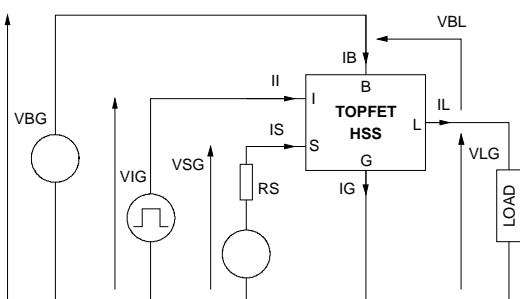
Fig.4. High side switch measurements schematic.
