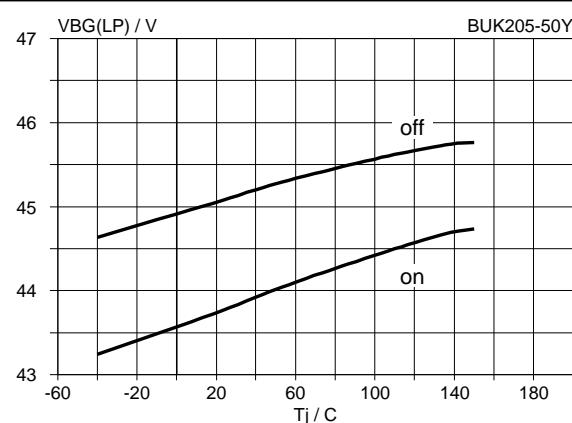
Fig.25. Supply typical overvoltage thresholds,  $V_{BG(LP)} = f(T_j)$ ; conditions  $V_{IG} = 5 V$ ;  $I_L = 80 mA$
