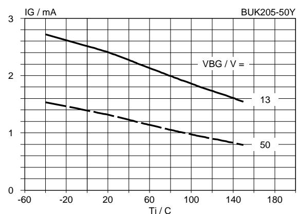
Fig.11. Typical operating supply current.
