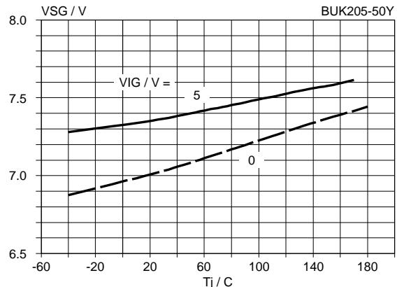
Fig.22. Typical status clamping voltage,  $V_{SG} = f(T_j)$ ; parameter  $V_{IG}$ ; conditions  $I_S = 100 \mu A$ ,  $V_{BG} = 13 V$
