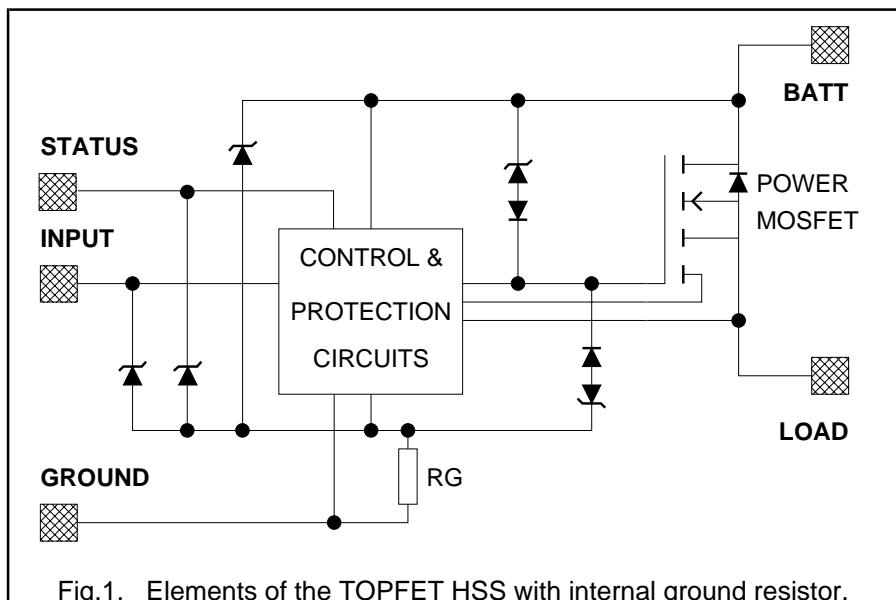
Fig.1. Elements of the TOPFET HSS with internal ground resistor.
