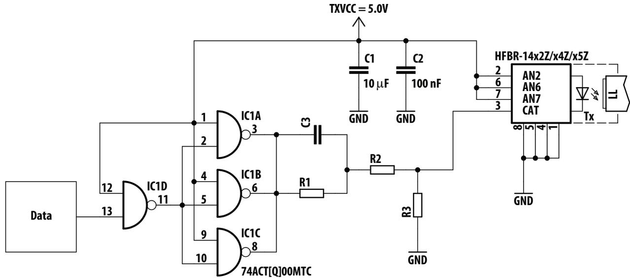
Note: The component values shown in the table create a typical driver current of 60mA (peak).
