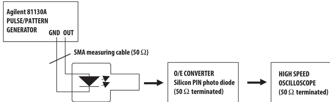
Figure 12. Test Circuit for Measuring  $t_r$ ,  $t_f$
