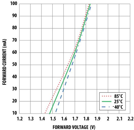
Figure 9. Typical Forward Voltage and Current Characteristics
