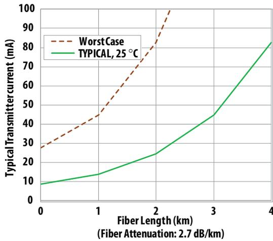
Figure 5. Typical HFBR-14x4xZ/HFBR-24x2xZ Link with 50/125  $\mu\text{m}$  Fiber
