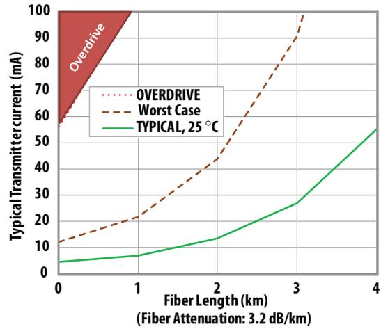
Figure 4. Typical HFBR-14x4xZ/HFBR-24x2xZ Link with 62.5/125  $\mu\text{m}$  Fiber
