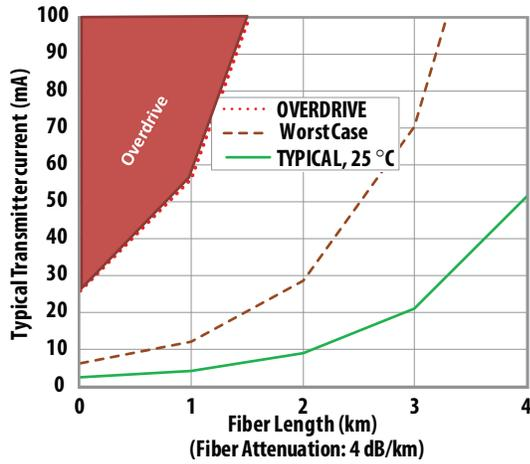
Figure 3. Typical HFBR-14x4xZ/HFBR-24x2xZ Link with 100/140  $\mu\text{m}$  Fiber
