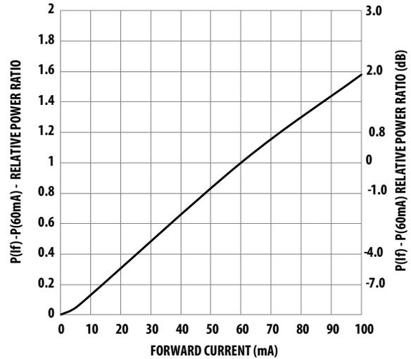
Figure 10. Normalized Typical Transmitter Output vs. Forward Current
