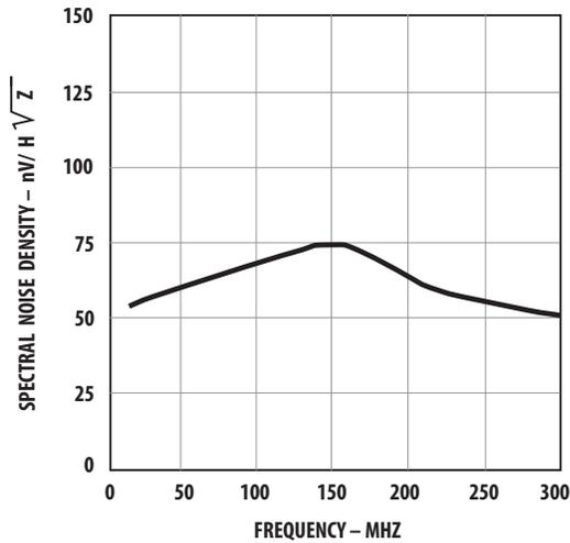
Figure 15. Typical Spectral Noise Density vs. Frequency
