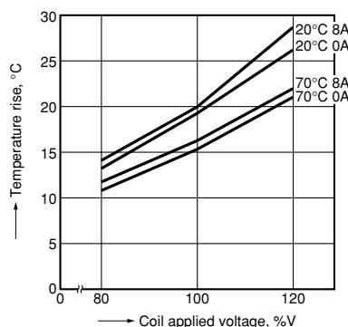
**3-(1). Ambient temperature characteristics and coil applied voltage (TV-5 type)**
