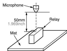
When operate (At contact making)
