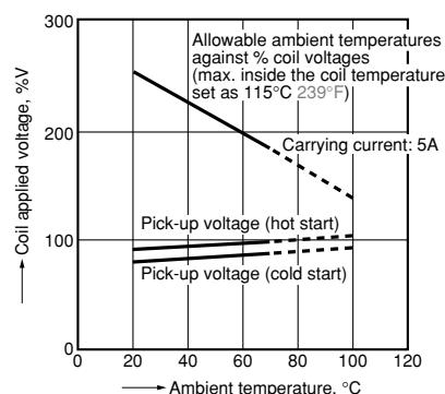
**3-(2). Ambient temperature characteristics and coil applied voltage (TV-8 type)**
