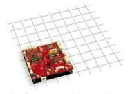
The Raven combines mid performance Atom Bay Trail processing with extensive on-board I/O in a compact 95 x 95 mm package!
