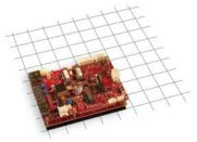
The Blackbird provides very high performance in a compact 95 x 125mm footprint. Featuring the Intel Skylake CPU, both dual and quad core versions are available with high performance video processing.
