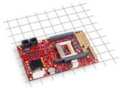
The Newt leverages the DMP Vortex86DX processor for low power/lower performance operation in a medium-sized format.
