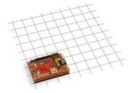
The Hawk is designed around the Intel Bay Trail CPU and features a moderate amount of on-board I/O. It is available in single, dual, and quadcore models to match the performance and power needs of each application.
