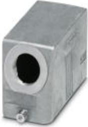
Sleeve housing B16, for single locking latch, Material: Die-cast aluminum, salt water resistant, Cable outlets: 1, lateral, Height: 60 mm, Cable gland: none, Gland: no, 1x Pg21, Standard
