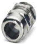
Cable gland, Cable gland material: Brass, nickel-plated, External cable diameter 13 mm ... 18 mm, Shielding: No, Connecting thread: Pg21, Color: silver
