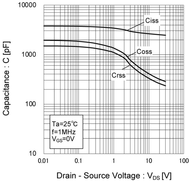
Fig.18 Switching Characteristics
