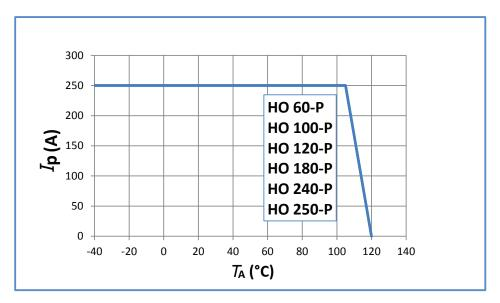
Important notice: whatever the usage and/or application, the transducer primary bar / jumper temperature shall not go above the maximum rating of 120 °C as stated in page 2 of this datasheet.
