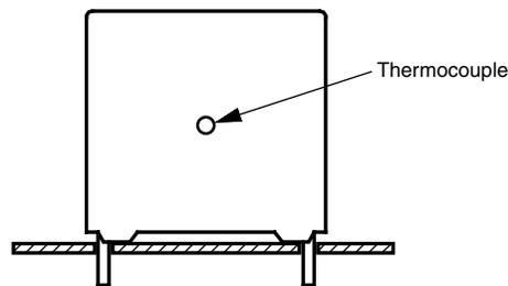
The temperature is measured in unloaded ( $T_{\text{amb}}$ ) and maximum loaded condition ( $T_C$ ).
