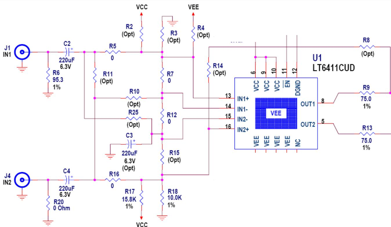
Figure 3. Input and Output Networks of the DC1108 Demo Board
