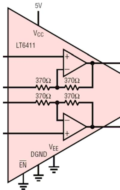
Figure 2. Block Diagram of LT6411 Internal Amplifiers and Resistors
