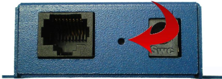
Figure 2. *Mode/Reset Switch*
