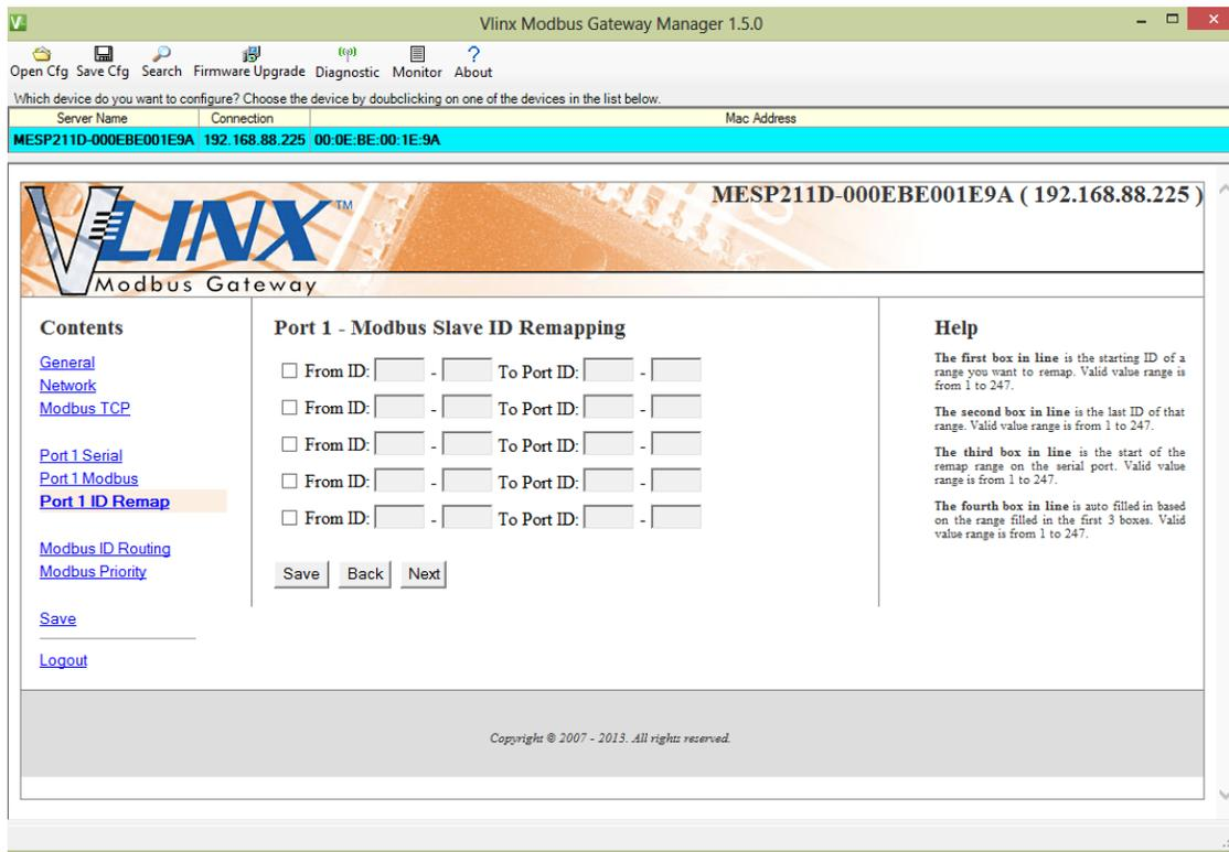
Figure 49. Port 1 Modbus Slave ID Remapping
