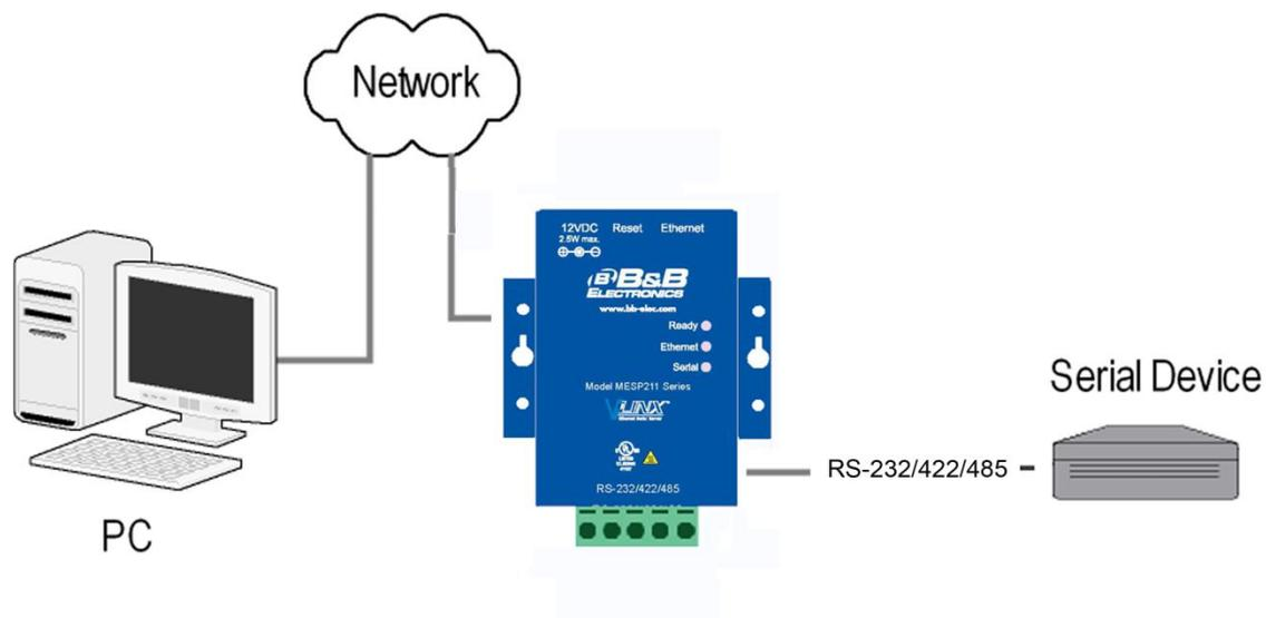
Figure 11. MESP211 Connections
