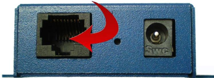
Figure 3. *Ethernet Connector.*
