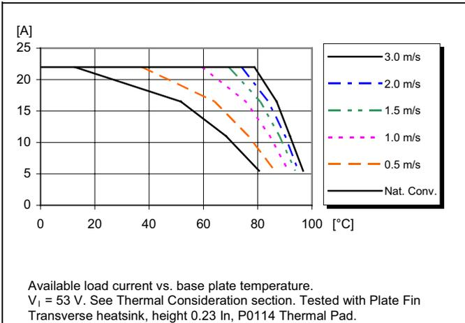
**Output Current Derating – Cold wall sealed box**
