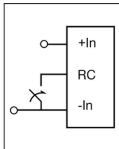
voltage generated on the RC pin is max 6 V. The standard product is provided with "negative logic" remote control and will be off until the RC pin is connected to the -In. To turn on the product the voltage between RC pin and -In should be less than 1 V. To turn off the product the RC pin should be left open for a minimum of time 150  $\mu$ s, the same time requirement applies when the product shall turn on. In situations where it is desired to have the product to power up
