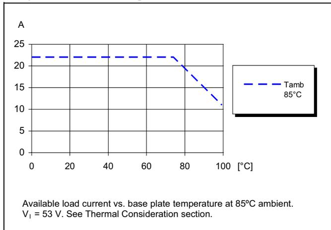
**Electrical Specification****12 V, 25 A, 300 W** $T_{p1} = -40$  to  $+90^{\circ}\text{C}$ ,  $V_i = 40$  to  $60$  V.Typical values given at:  $T_{p1} = +25^{\circ}\text{C}$ ,  $V_i = 53$  V,  $I_o = \text{max } I_o$ , unless otherwise specified under Conditions.Additional  $C_{out} = 0.1$  mF. See Operating Information section for selection of capacitor types.
