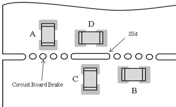
Stress strength according to the mounting position:
