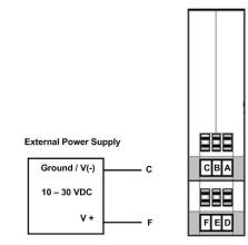
Current Loop Converter uses 2.5 W
