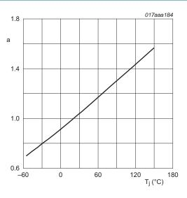
$$a = \frac{R_{DSon}}{R_{DSon(25^{\circ}C)}}$$
