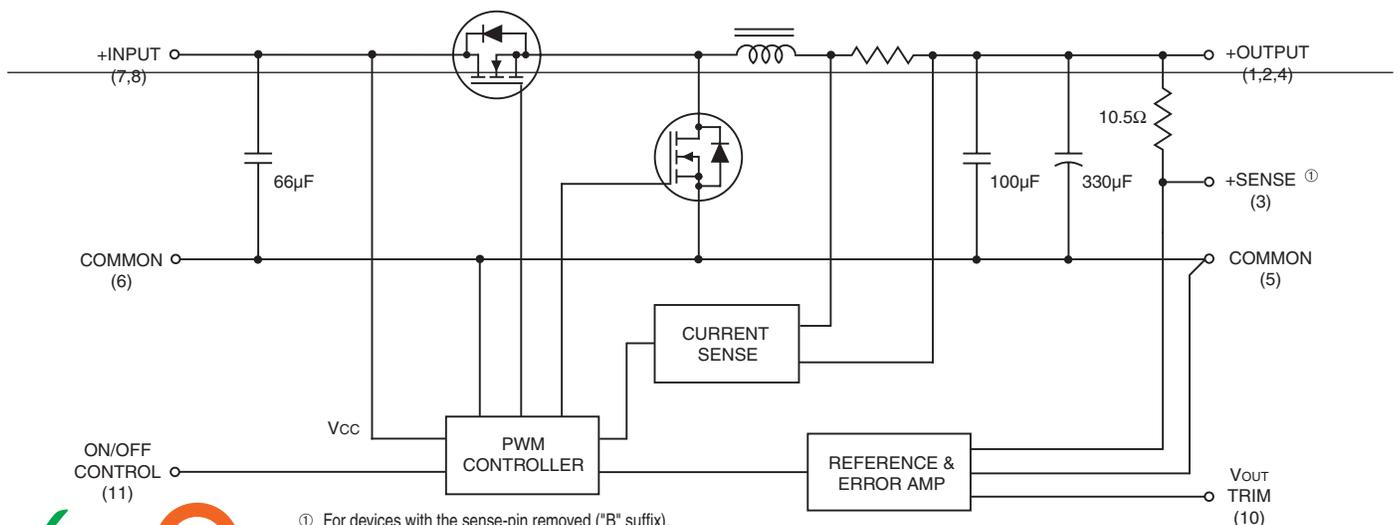
① For devices with the sense-pin removed ("B" suffix), the feedback path is through the +Output pin and not the +Sense pin.
