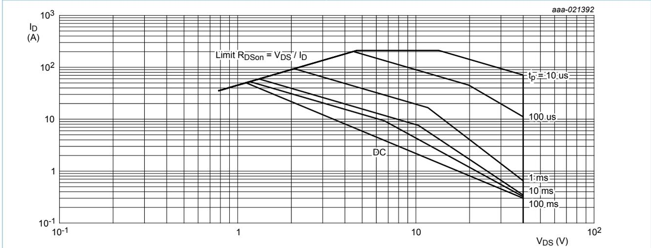
$T_{mb} = 25 \text{ }^\circ\text{C}$ ;  $I_{DM}$  is a single pulse
