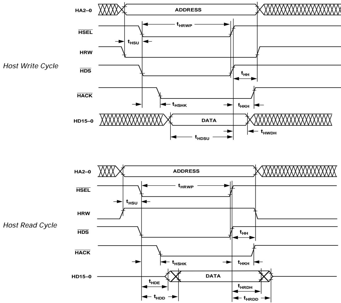
Figure 36. Host Interface Port (HMD1 = 0, HMD0 = 1)
