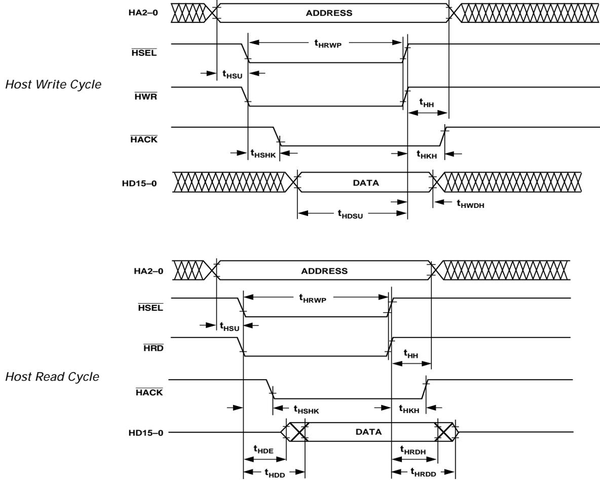
Figure 35. Host Interface Port ( $HMD1 = 0$ ,  $HMD0 = 0$ )
