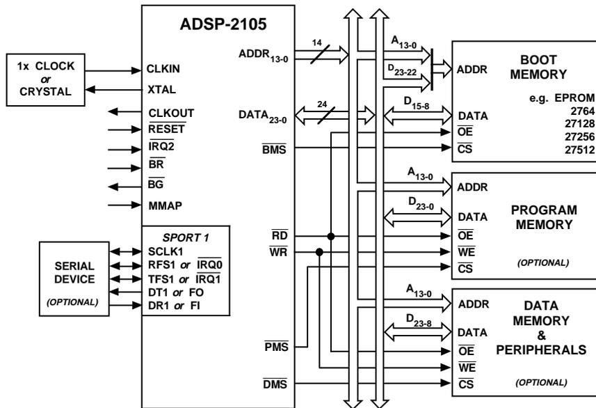
THE TWO MSBs OF THE DATA BUS (D<sub>23-22</sub>) ARE USED TO SUPPLY THE TWO MSBs OF THE BOOT MEMORY EPROM ADDRESS. THIS IS ONLY REQUIRED FOR THE 27256 AND 27512.
