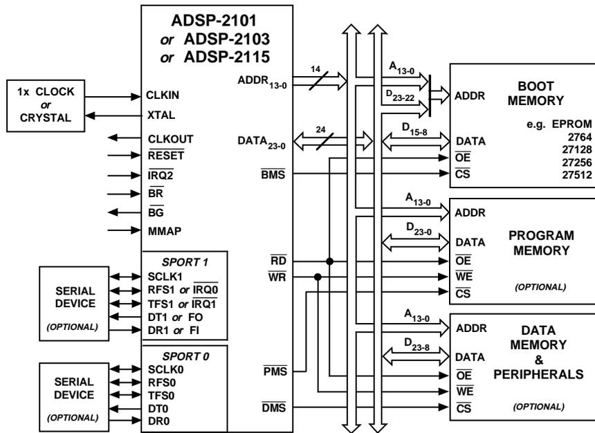
THE TWO MSBs OF THE DATA BUS (D<sub>23-22</sub>) ARE USED TO SUPPLY THE TWO MSBs OF THE BOOT MEMORY EPROM ADDRESS. THIS IS ONLY REQUIRED FOR THE 27256 AND 27512.
