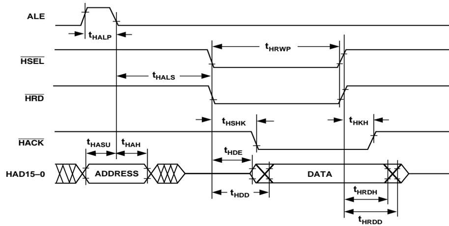
Figure 37. Host Interface Port (HMD1 = 1, HMD0 = 0)
