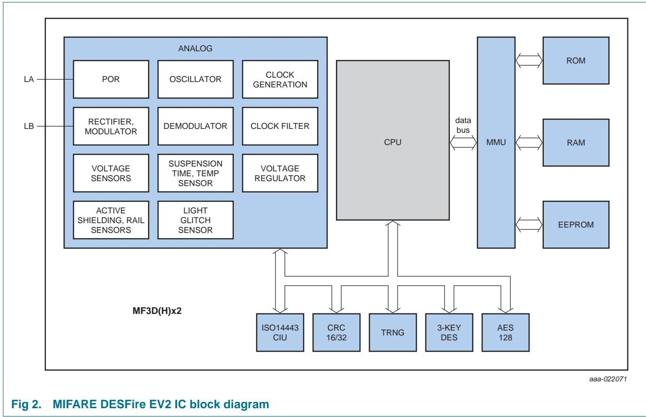
**Fig 2. MIFARE DESFire EV2 IC block diagram**
