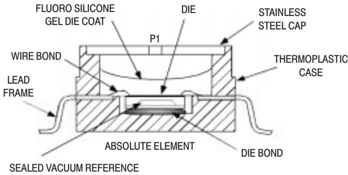
**Figure 2. Cross Sectional Diagram SOP (not to scale)**
