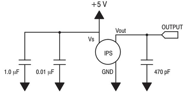
**Figure 3. Recommended power supply decoupling and output filtering.**
