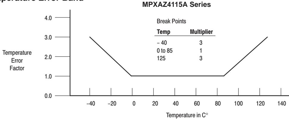
NOTE: The Temperature Multiplier is a linear response from 0°C to -40°C and from 85°C to 125°C
