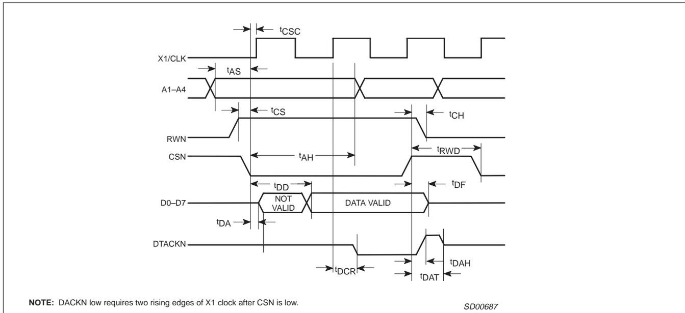
**Figure 6. Bus Timing (Read Cycle) (68XXX mode)**
