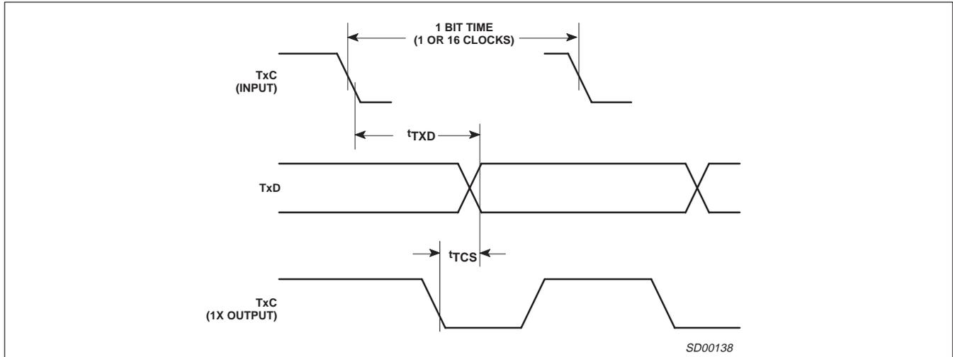
Figure 12. Transmitter External Clocks
