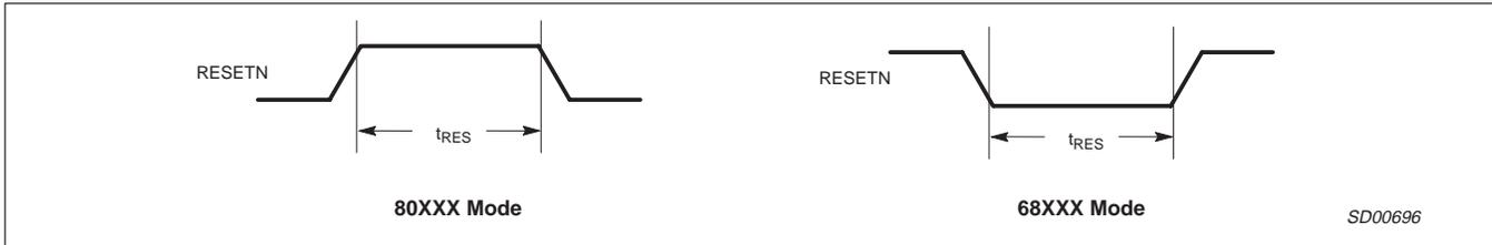
Figure 4. Reset Timing
