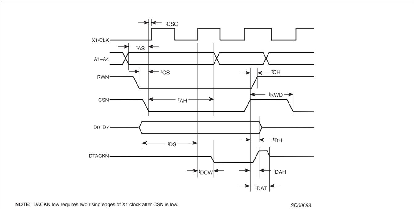
**Figure 7. Bus Timing (Write Cycle) (68XXX mode)**
