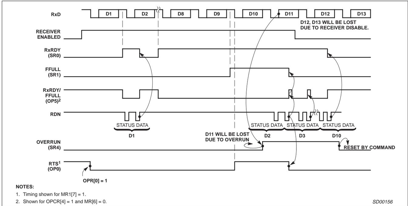
Figure 15. Receiver Timing
