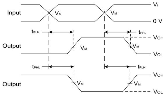
**Voltage Waveform Propagation Delay Times
