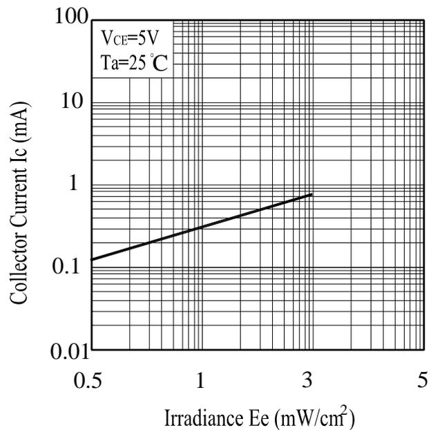
**Typical Electro-Optical Characteristics Curves**
