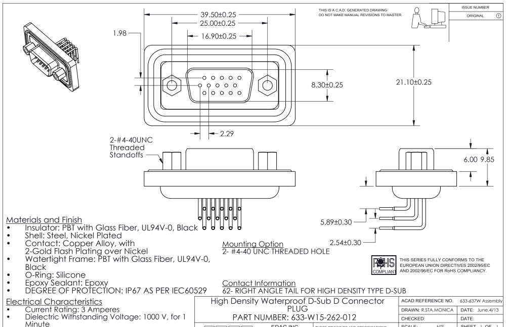
Insulation Resistance: 5000 Megohm Min. Contact Resistance: 10 Milliohms Max.
