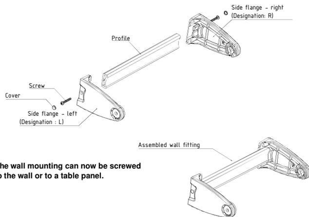
The wall mounting can now be screwed to the wall or to a table panel.
