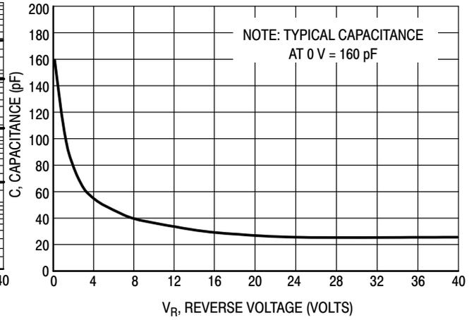
Figure 4. Typical Capacitance
