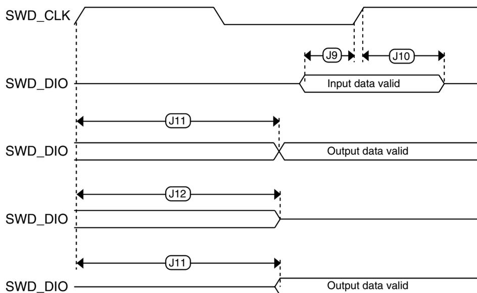
Figure 14. Serial wire data timing
