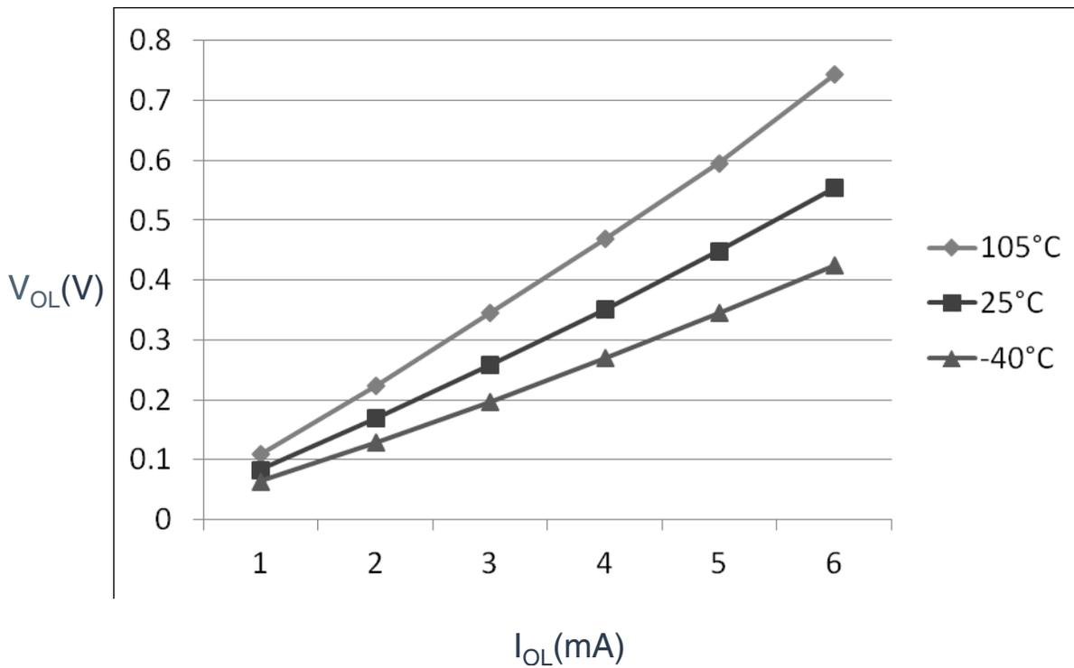
Figure 6. Typical V<sub>OL</sub> Vs. I<sub>OL</sub> (standard drive strength) (V<sub>DD</sub> = 3 V)
