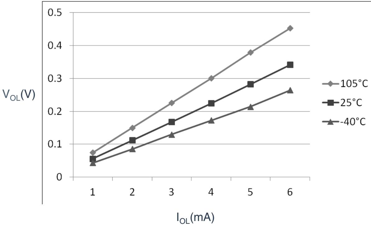
Figure 5. Typical V<sub>OL</sub> Vs. I<sub>OL</sub> (standard drive strength) (V<sub>DD</sub> = 5 V)
