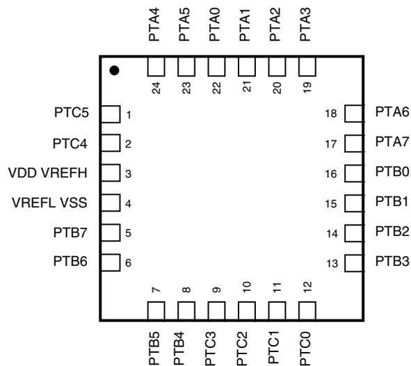
**Figure 21. 24-pin QFN package**
