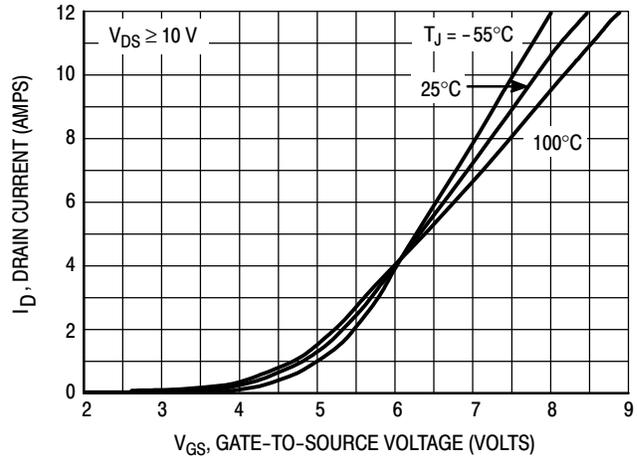
Figure 2. Transfer Characteristics
