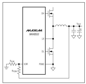
Figure 5. Setting the Foldback Current Limit with Two Resistors, RJLIM and RFOBK
