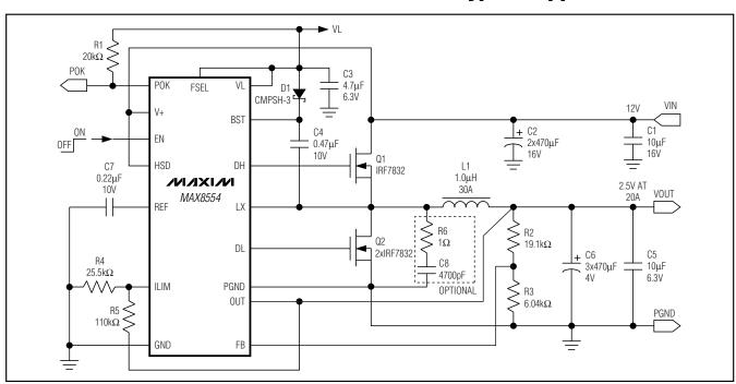
Figure 1. Typical Application Circuit 1: 12V Input, 2.5V Output at Up to 20A with 200kHz Switching Frequency
