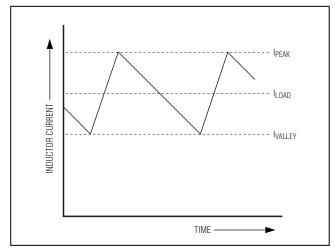
Figure 4. Inductor-Current Waveform
