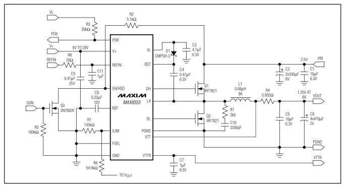
Figure 2. Typical Application Circuit 2: 2.5V Input, 1.25V VTT at Up to 8A, and 1.25V VTTR at Up to 25mA with 550kHz Switching
