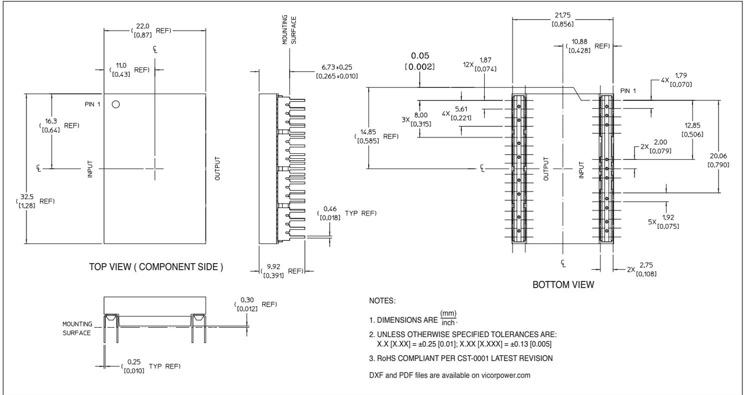
Figure 12 — VTM™ through-hole module mechanical outline
