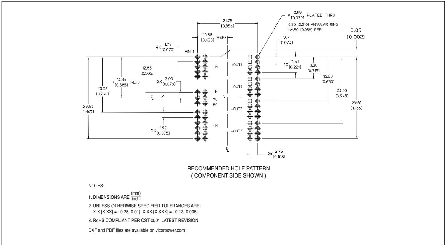
Figure 13 — VTM™ through-hole module PCB layout information
