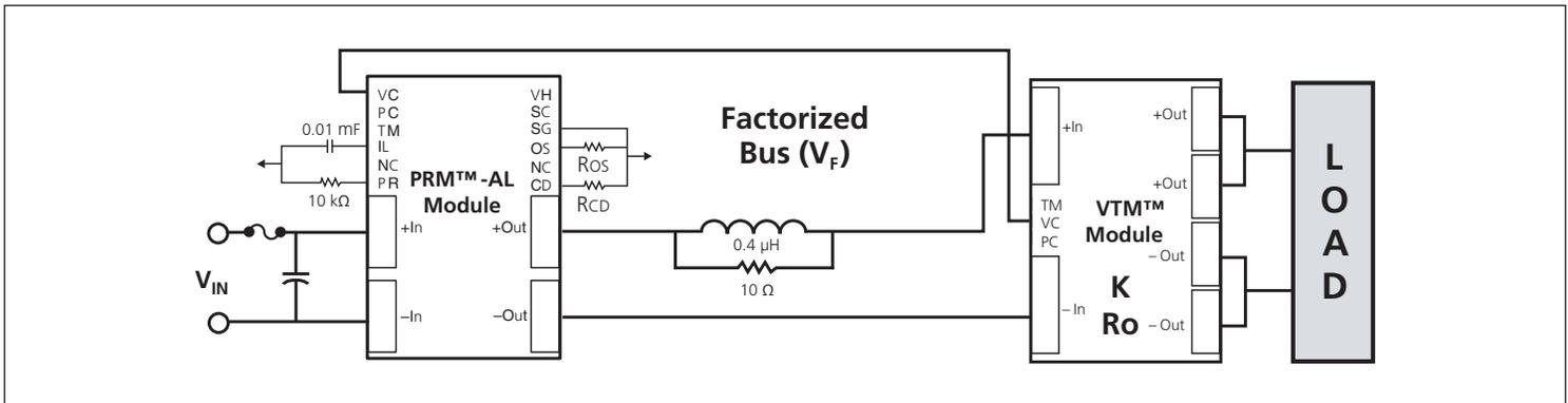
**Figure 18** — The PRM™ regulator controls the factorized bus voltage, V<sub>F</sub>, in proportion to output current to compensate for the output resistance, R<sub>O</sub>, of the VTM™ current multiplier. The VTM module output voltage is typically within 1% of the desired load voltage (V<sub>L</sub>) over all line and load conditions.
