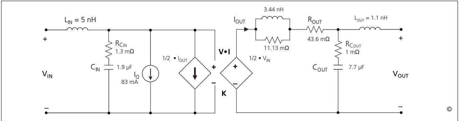
**Figure 17** — This model characterizes the AC operation of the V•I Chip VTM including response to output load or input voltage transients or steady state modulations. The model enables estimates or simulations of input and output voltages under transient conditions, including response to a stepped load with or without external filtering elements.
