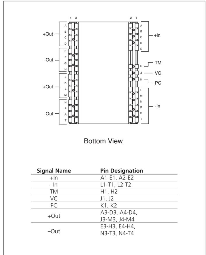
Figure 9 — VTM™ current multiplier pin configuration
