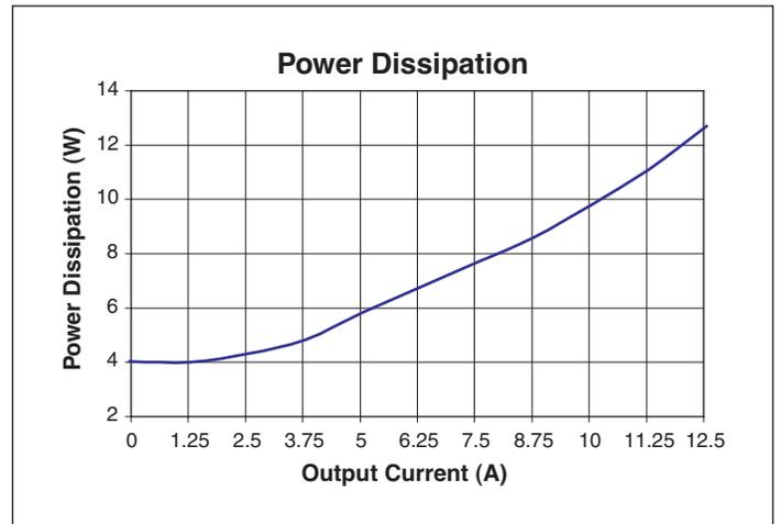
Figure 4 — Power dissipation vs. output current.
