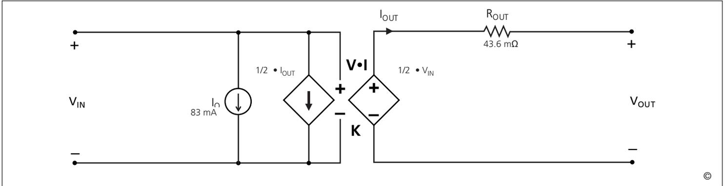
**Figure 16** — This model characterizes the DC operation of the V•I Chip VTM, including the converter transfer function and its losses. The model enables estimates or simulations of output voltage as a function of input voltage and output load, as well as total converter power dissipation or heat generation.
