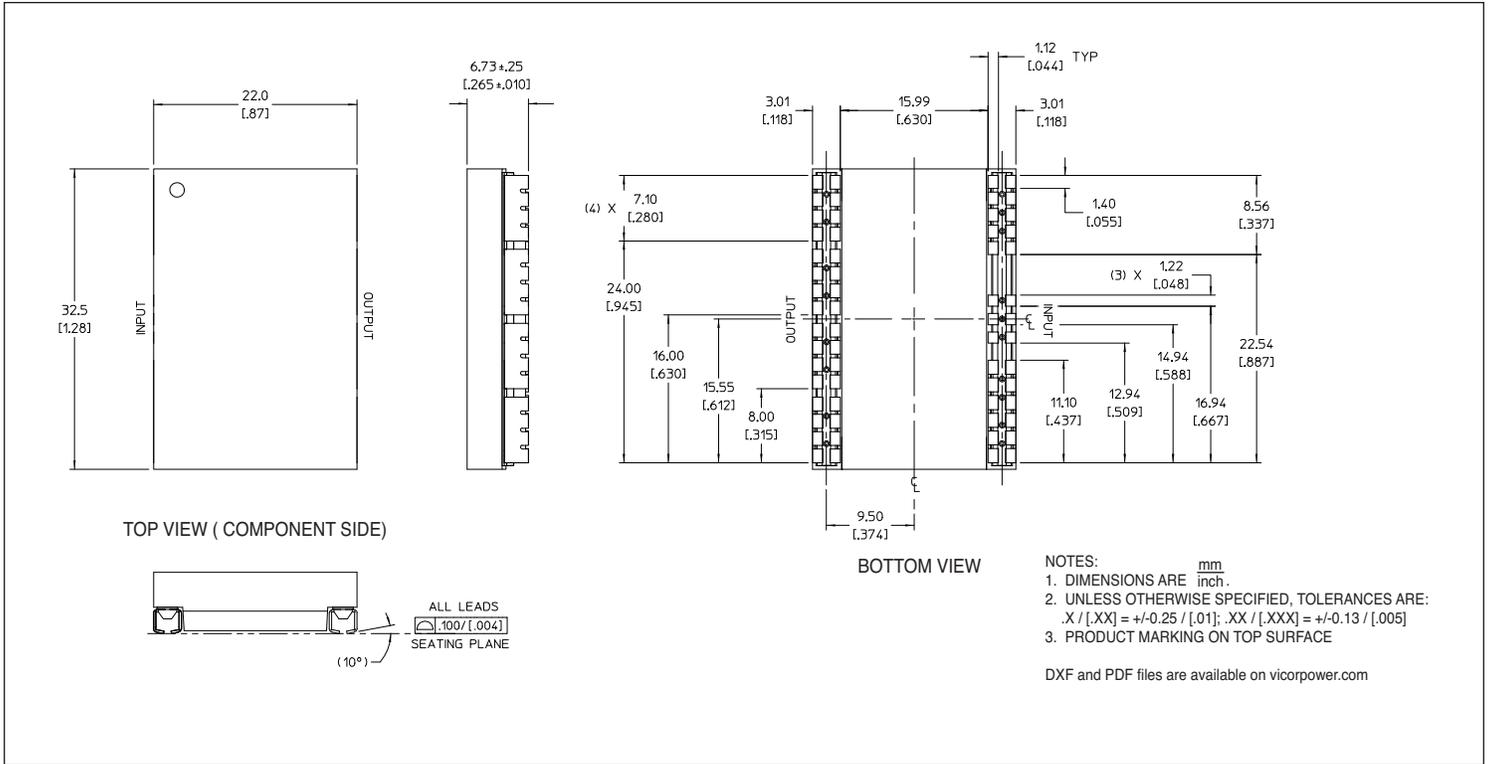
Figure 10 — VTM™ module J-Lead mechanical outline; Onboard mounting
