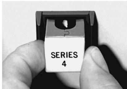
1. Lamps and legends can be changed from panel front. When button is removed, lamp is extracted from its socket and retained in button.
